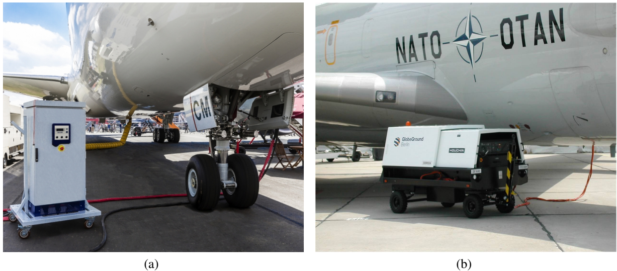
Figure 6.1: (a) Power Electronics based GPU and (b) Diesel operated GPU.
