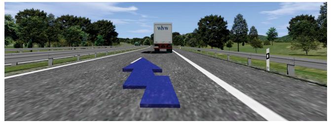
(b) Contact-analog arrow, indicating best overtake time
