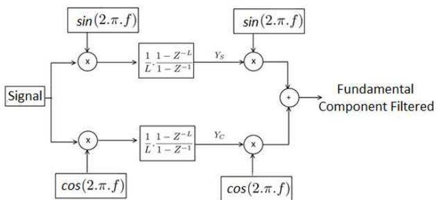
Fig. 6. Filter structure based on SWRDFT.
