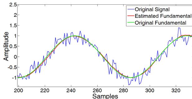
Fig. 7. Result of the filtered fundamental component utilizing the SWRDFT filter.
