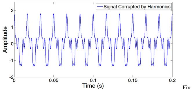
Fig. 9. Signal corrupted by third (50% energy) and sixth (30% energy) harmonics.
