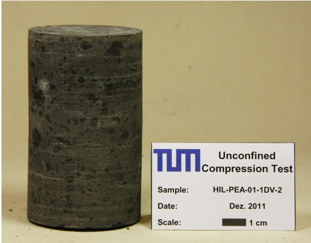
Fig. 47: Specimen of a kimberlite rock of the mine Peakstar. Sample HIL-PEA-01.
