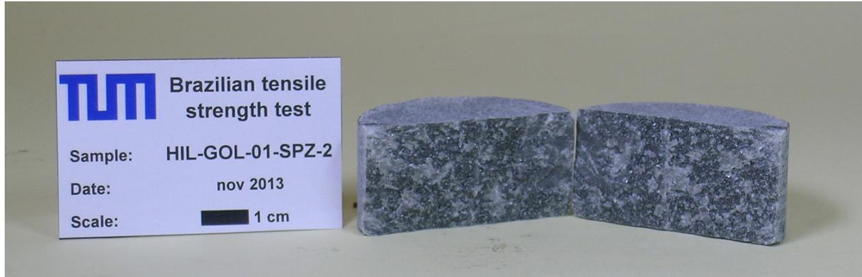
Fig. 57: Picture of a Brazilian test sample of the Golling anhydrite. Sample HIL-GOL-01.
