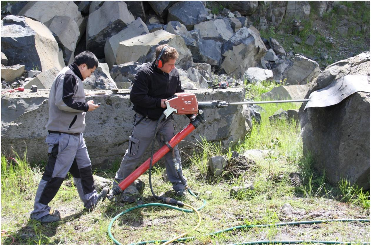
Fig. 37: Field drill testing in progress. One person is drilling and the second one is registering the drilling time for each hole.
