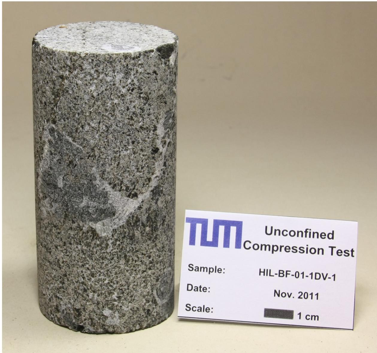
Fig. 45: Specimen of pyroxenite as an example for all considered platinum samples. HIL-BRA-01.
