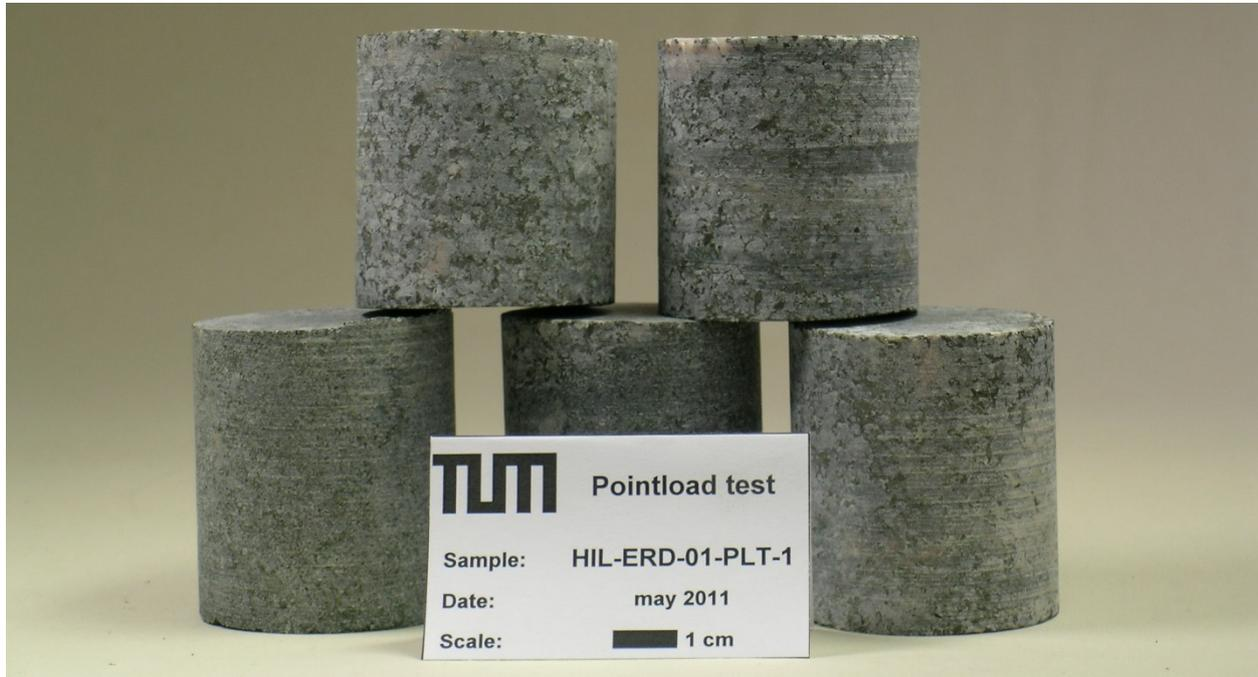
Fig. 55: Picture of point load samples of the Erdösmecke granite. Sample HIL-ERD-01.
