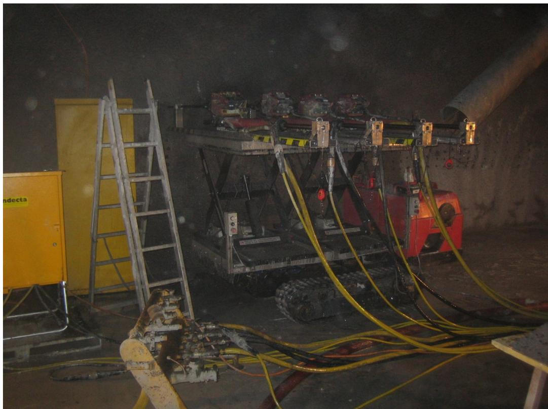
Fig. 35: In line drill test set-up with a drill rig at the Hagerbach Test Gallery (Switzerland) (Picture: Stefan Götzfried).
