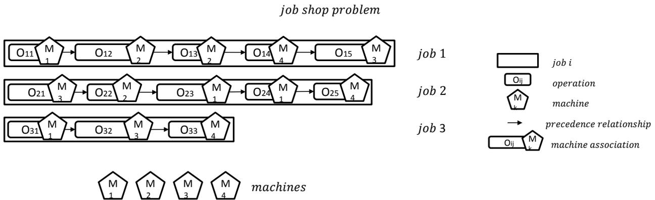
Figure 2-16: Schematic representation of a job shop problem: the jobs are made up of different ( $n_i$ ) amounts of operations ( $O_{ij}$ ) that are connected to each other with precedence relationships as described by the flow shop problem. For the job shop problem the ID of the required machine for a task’s execution is not necessarily equal to the task’s place in the flow sequence.
