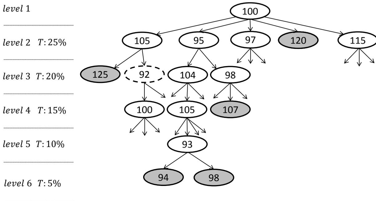
Figure 7-10: Schematic representation of the working mechanism of the simulated annealing algorithm to traverse through the solutions of the enumeration tree. Grey node: fathomed, dashed ellipse: current best solution, arrows: applied swaps, T: tolerance factor at the corresponding level
