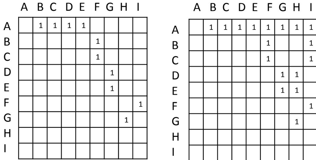
Figure 5-11: Adjacency matrix (left) and the transitive closure (right) of the introduced precedence graph (Figure 5-10)
