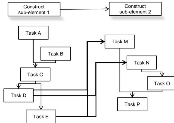
Figure 4-8: The process of mapping high-level precedence-constraints to the task-level: set a new constraint between all the tasks of the predecessor component that have no successor within the component (task D, E) as precedence of all the tasks in the successor component without predecessor within the component (task M,N)
