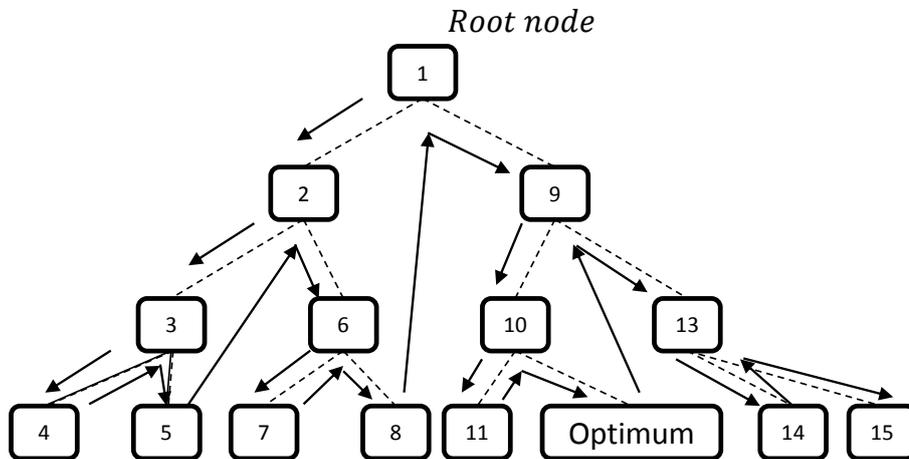
Figure 6-11: Schematic representation of the working mechanism of the depth first search without fathoming any nodes (numbers: order of determination)
