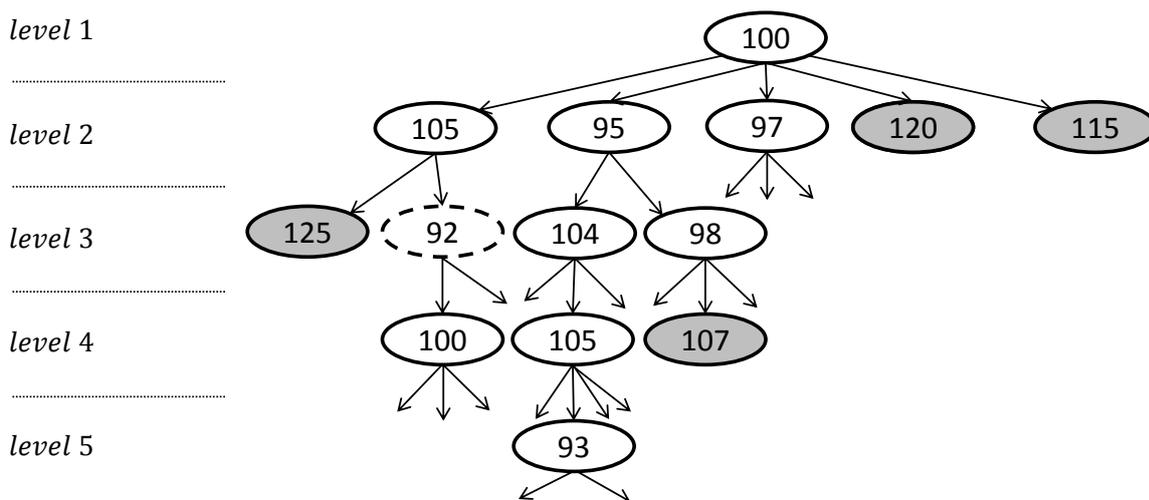
Figure 7-9: Schematic representation of the greedy-like heuristic algorithm. Grey: Fathomed nodes, dashed ellipse: current best solution, arrows: applied greedy heuristic. Tolerance factor: 15%.
