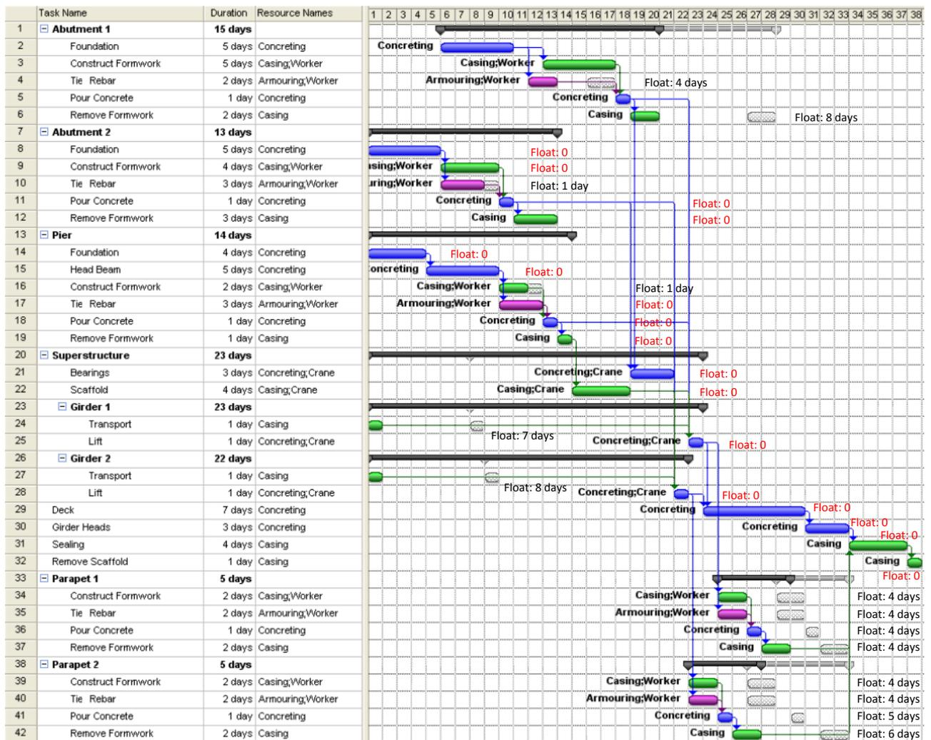
Figure 5-23: Results of the float time calculation after introducing further resource constraints to the project
