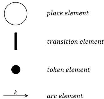
Figure 3-20: Modeling elements of a Petri Net
