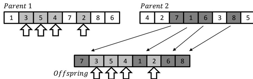
Figure 6-21: Position-based cross over: chromosomes made up of eight components that represent task IDs from a schedulable project. The selected component of the first parent (light grey) will be inserted into the offspring at the same position. The missing element will be filled up from the second parent (dark grey) keeping the sequence of the components.
