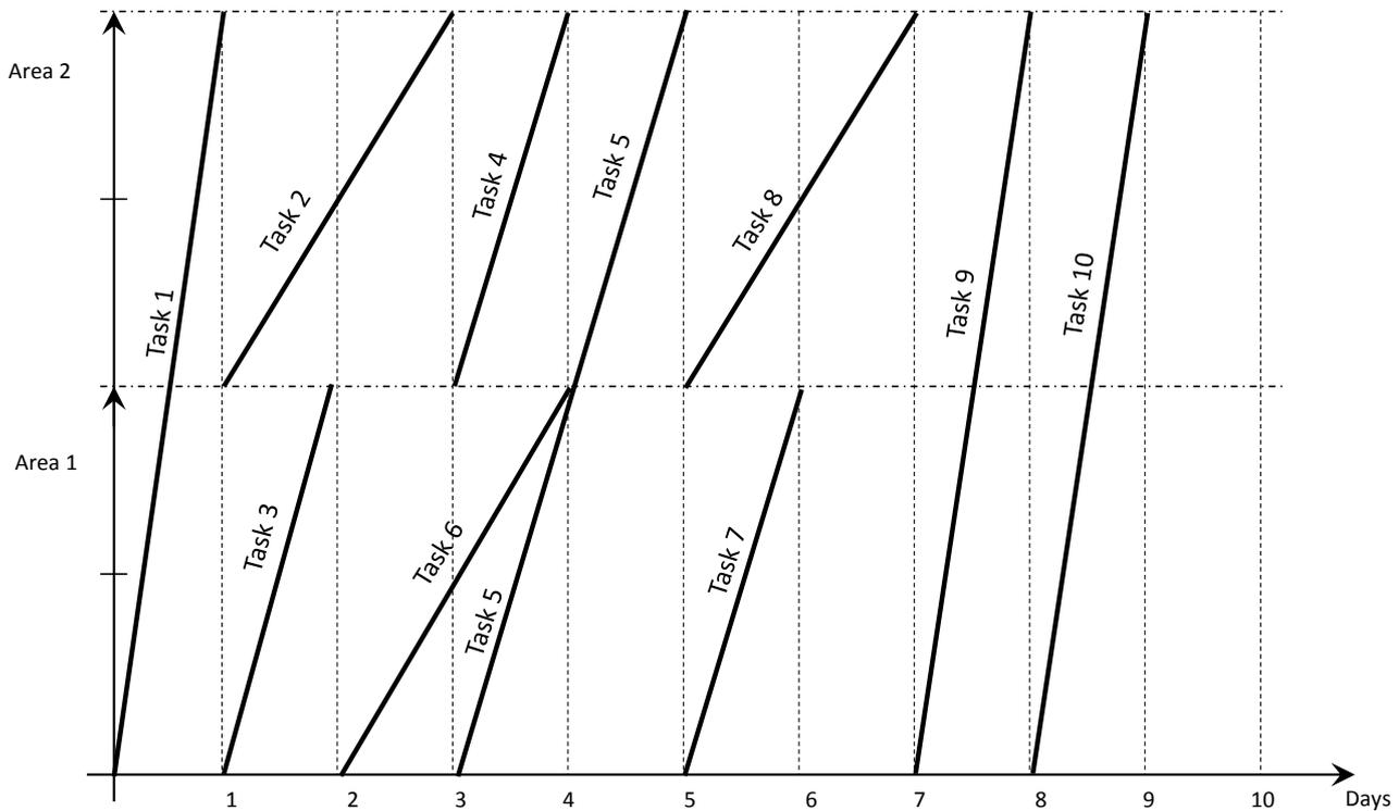
Figure 2-4: Linear schedule representation of the introduced construction project from Figure 2-1. The construction site is divided into two regions: area 1 and area 2. The execution direction of every task is forward from the start point to the end of area two. There are tasks, such as task1, task 5, task 9 and task 10, which are executed continuously in both areas and the other tasks that are executed only in one area (e.g. task 2 in area 2 and task 3 in area 1).
