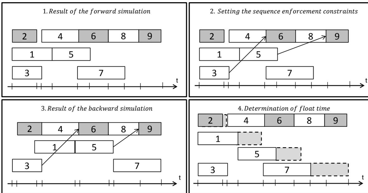
Figure 5-15: Determination of the sequence enforcement constraints for the backward simulation after the forward simulation. (Different colors: different resource needs, arrows: new constraints, dashed boxes: float time)
