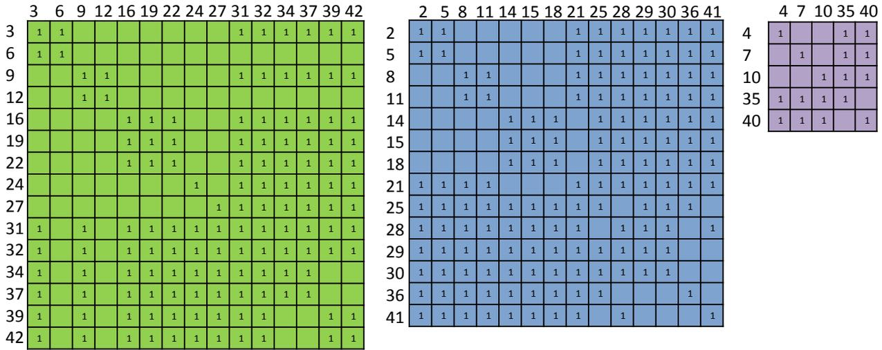
Figure 5-20: The fragmented dependency matrices of the resource classes used for the test case. 1: dependent tasks, empty cell: independent tasks, green: “casing”, blue: “concreting”, purple: “armouring”.
