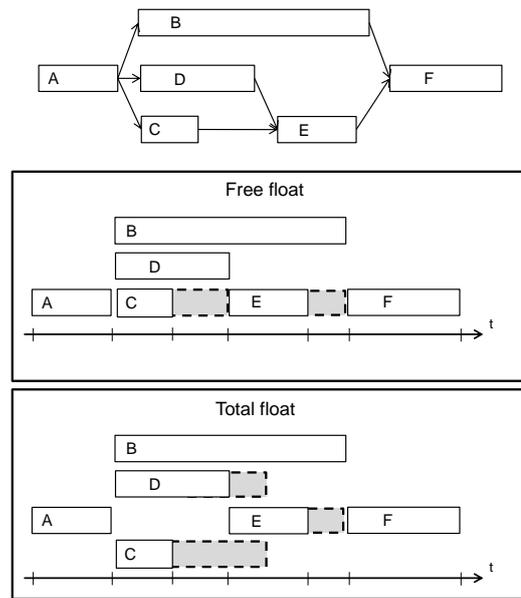
Figure 5-1: Difference between the free and the total float (top: precedence graph of the tasks, middle: free float, bottom: total float, dashed box: float)
