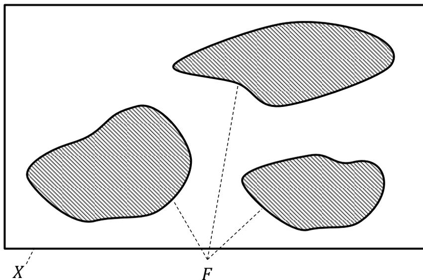
Figure 6-2: The solution space  $X$  and the fragmented feasible solution space  $F$  for a 2 dimensional space. The space inside  $X$  and outside of  $F$  represents the non-feasible solutions.
