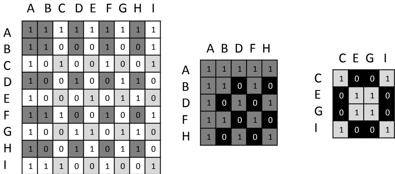
Figure 5-12: The dependency matrix and the fragmented dependency matrices for the different resource classes (dark and light gray). Black elements with white text: independent pair of tasks
