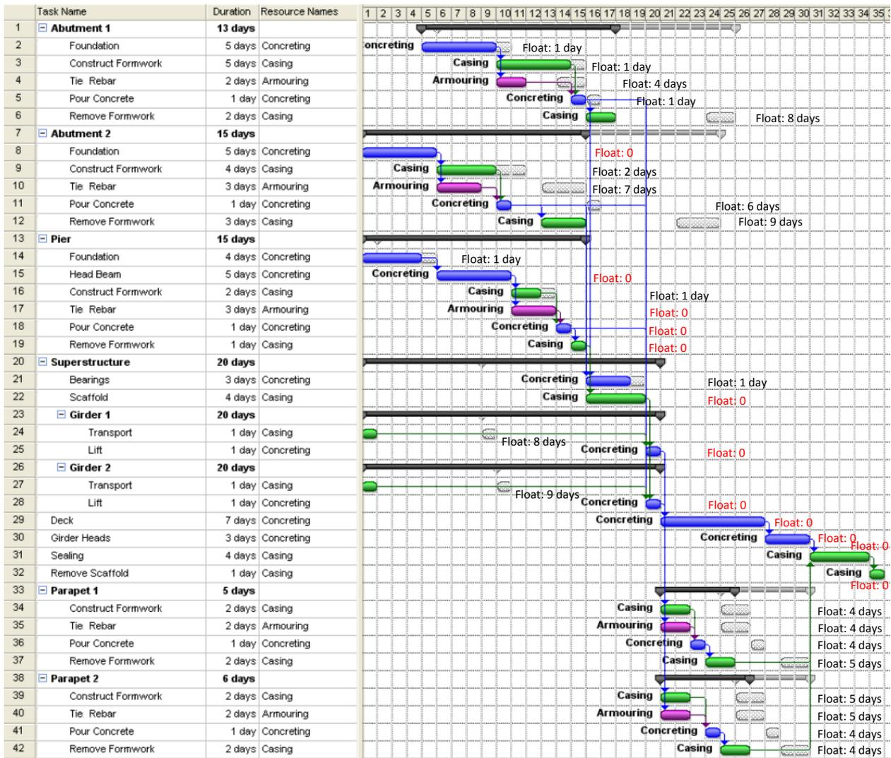
Figure 5-22: The expected result of the float time determination (created manually)
