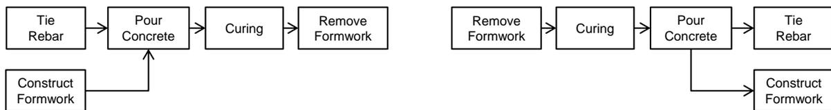
Figure 5-7 Precedence relationships for forward simulation (left) and for backward simulation (right)
