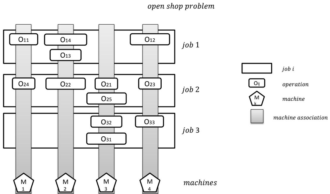
Figure 2-14: Schematic representation of an open shop problem example: the operations ( $O_{ij}$ ) of a  $job\ i$  have no precedence relationships between each other and are associated with one machine ( $M_k$ ) necessary for their execution.
