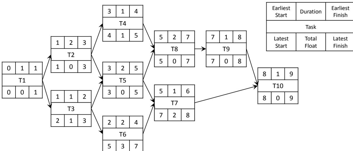
Figure 2-7: Activity-on-Node representation of the introduced construction project in Figure 2-1. Boxes: tasks, Arrows: precedence relationships. Information about the tasks like earliest or latest start time are represented inside the tasks box.
