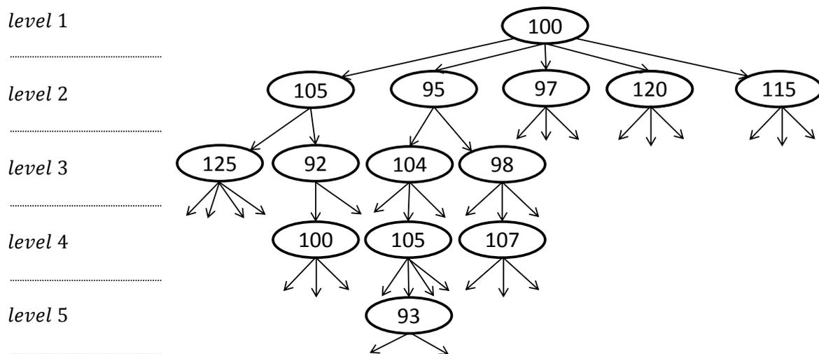
Figure 7-7: Schematic representation of a part of the enumeration tree. Every node symbolizes one schedule. On the top is level 1 representing a randomly generated base schedule. The number in the nodes represents the makespan of the schedule. One arrow accords to one applied reasonable priority swap.
