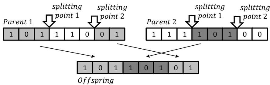
Figure 6-19: Two-point cross over: chromosomes made up of eight binary component. The components of the offspring are originated before the first splitting point and after the second one from the first parent (light grey), between them from the second parent (dark grey).
