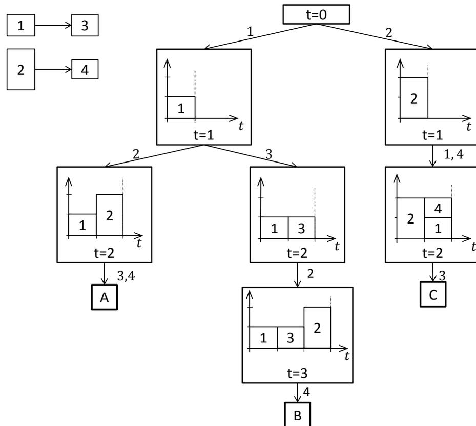
Figure 6-17: The Branch-and-Bound tree of the previous example determined by the extension alternatives
