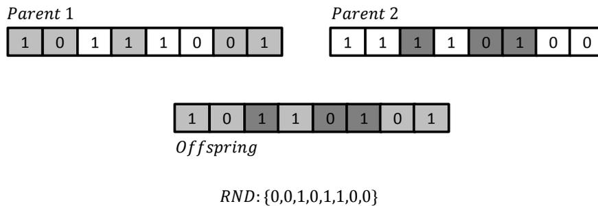
Figure 6-20: Uniform cross over: chromosomes made up of eight binary component. The components of the offspring are originated from the first parent (light grey) if the random value (RND) is zero, from the second parent (dark grey) results the random value if it is one.
