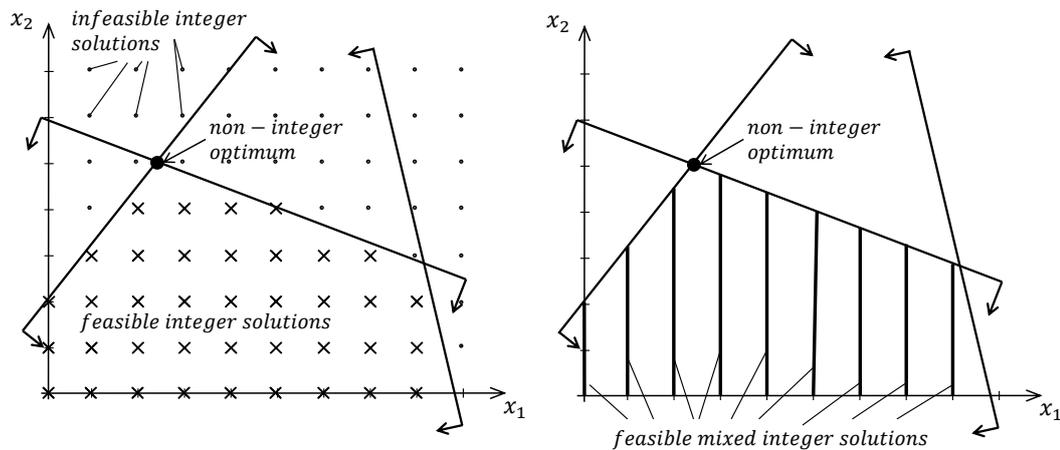
Figure 6-6: IP (left) and MIP (right) representation of the introduced two-dimensional problem (the feasible integer solutions are marked with X).
