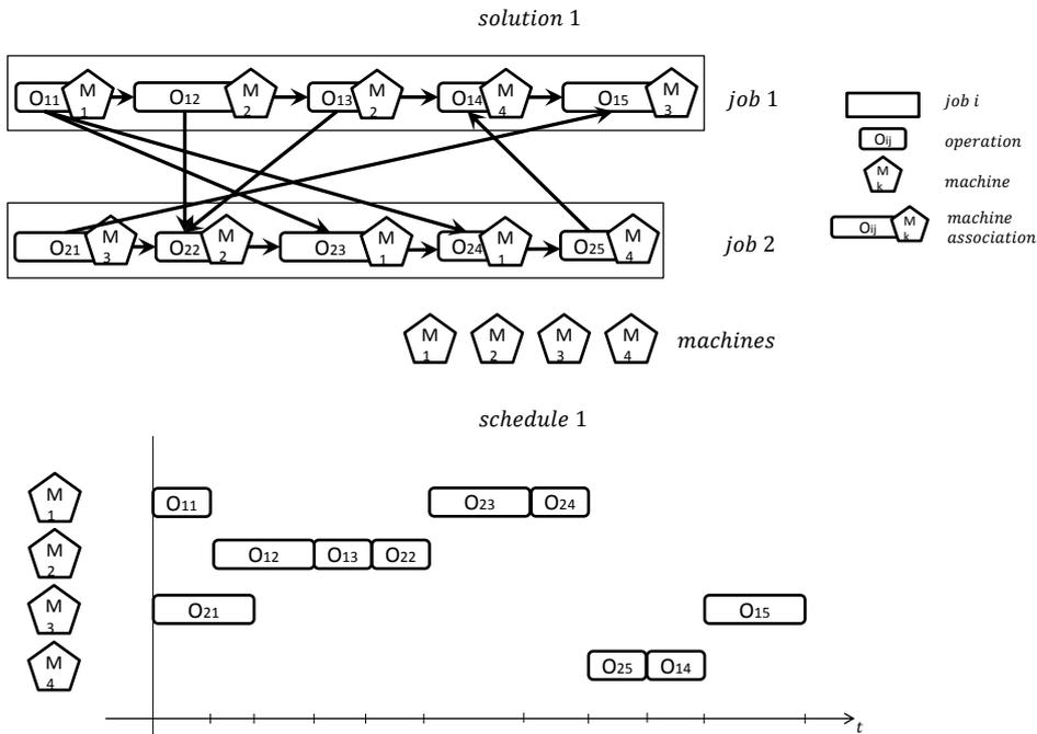
Figure 2-18: One feasible solution for the introduced disjunctive graph from Figure 2-17. Every disjunctive arc has been turned into a fixed arc resulting in an acyclic graph defining exact execution orders of the operations for every single machine.
