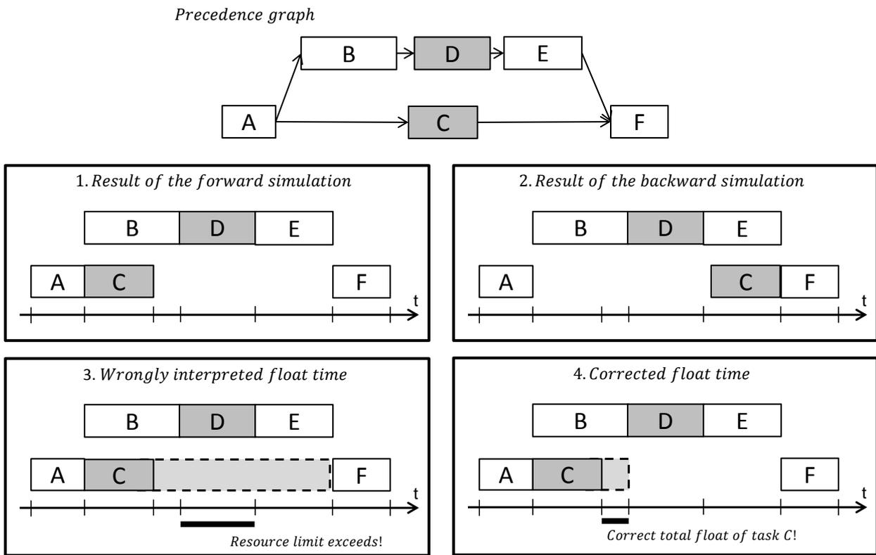
Figure 5-14: Results of the forward (1) and backward (2) simulations. The problem (3): exceeding the resource limits at the time period of float time. The solution (4): maintain the relative order of C and D → shorter total float time for C. (different colors: different resource needs)
