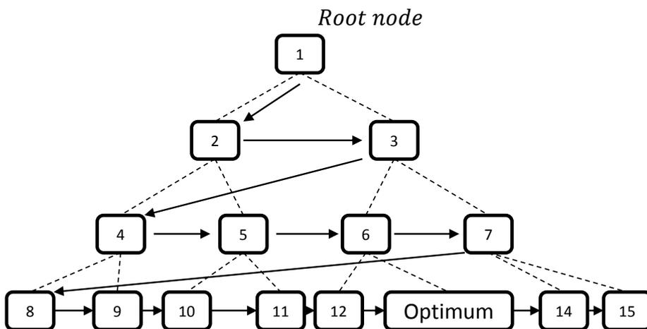
Figure 6-12: Schematic representation of the working mechanism of the breadth first search without fathoming any nodes (numbers: order of determination)
