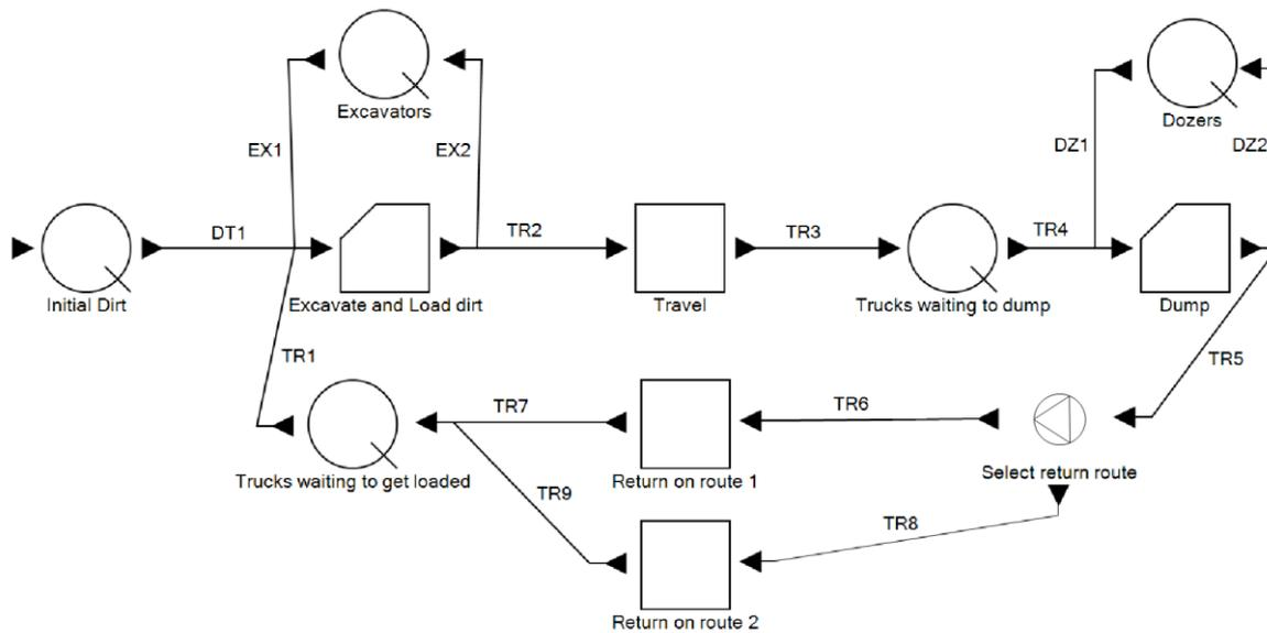
Figure 3-15: STROBOSCOPE ACD for the simple earthmoving system that was introduced in Figure 3-13 extended by a fork element allowing the trucks to select a return route. The meaning of link names: DT stands for dirt, EX for excavator, DZ for dozer and TR for truck.
