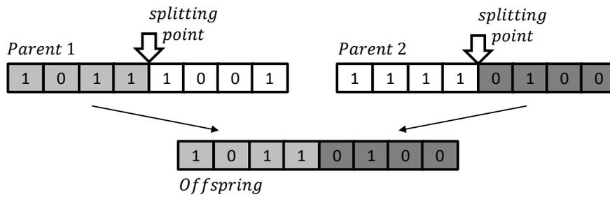
Figure 6-18: One-point cross over: chromosomes made up of eight binary components. The components of the offspring are originated before the splitting point from the first parent (light grey) and after that from the second parent (dark grey)
