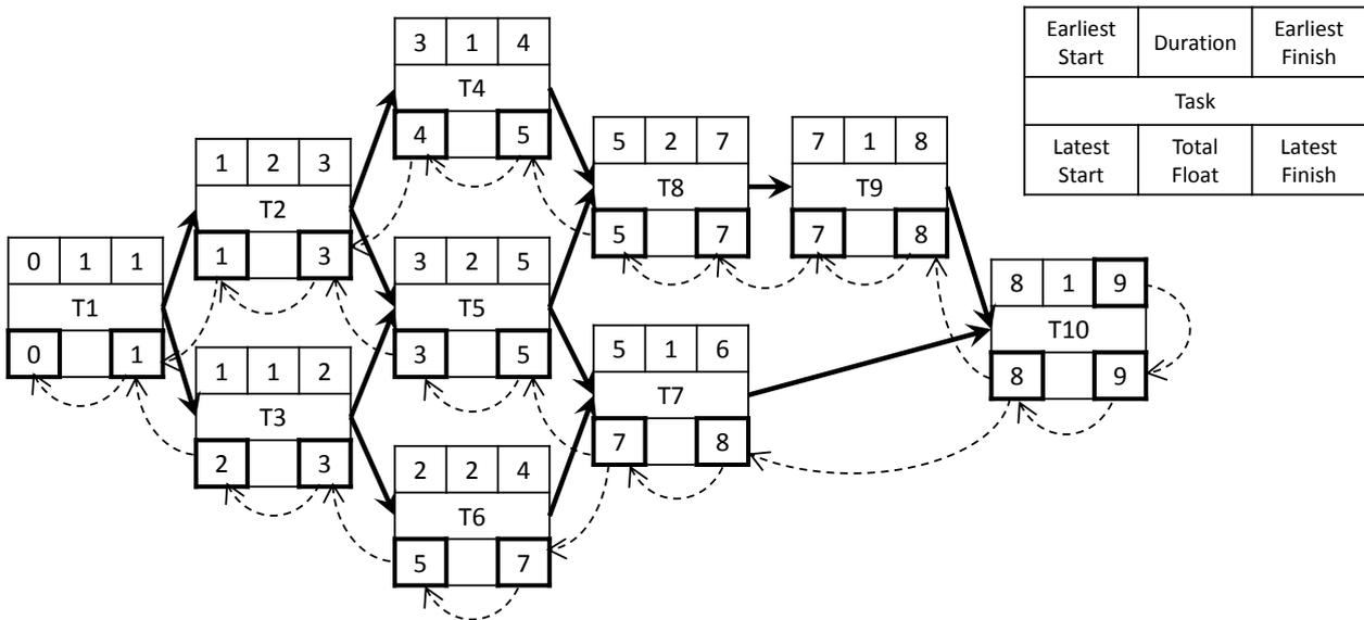
Figure 2-9: Schematic representation of the backward pass for the construction project introduced in Figure 2-1. Determination of the latest start and finish time of the tasks. Boxes: tasks, arrows: precedence relationships, dashed arrows: steps of the calculation.
