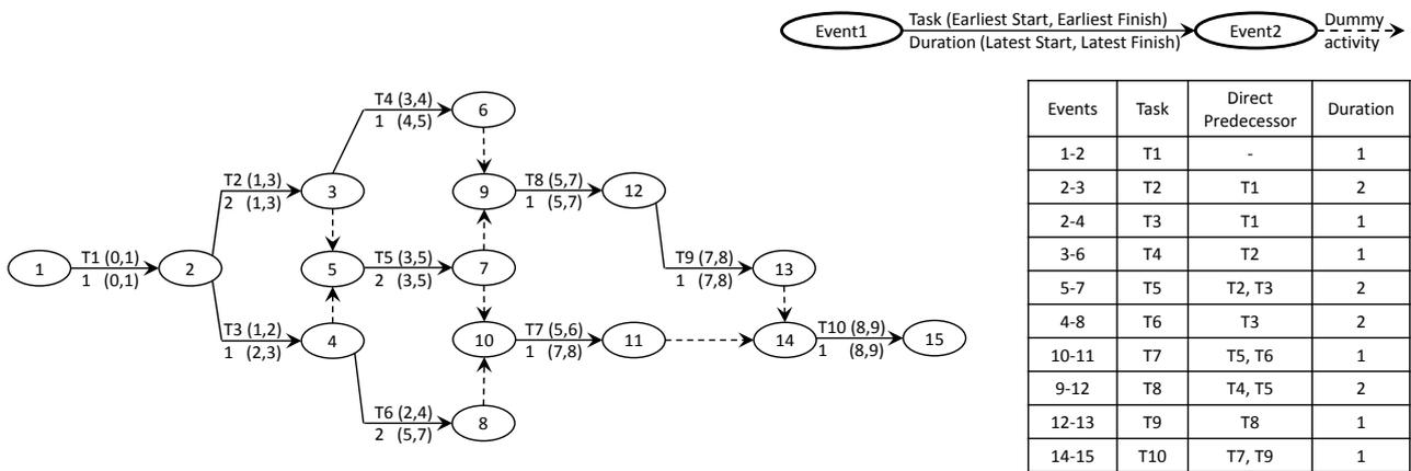
Figure 2-6: Activity-on-Arrow representation of the introduced construction project in Figure 2-1. Ellipses: Events, Arrows: tasks, dashed arrows: dummy activities.
