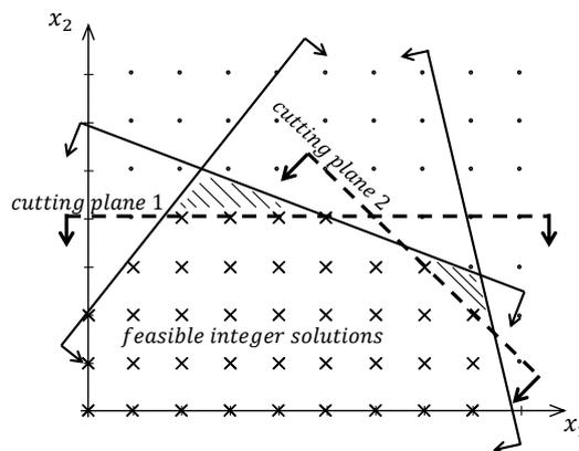
Figure 6-7: Cutting plane method: Cutting out bounding non-integer LP solutions so that every integer solution stays inside the considered solution space.
