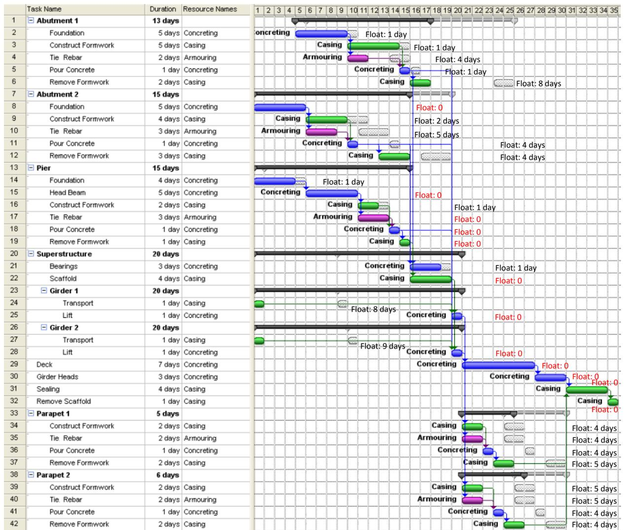
Figure 5-21: Feasible results of the forward and backward simulation using the priority-by-end-date method and sequence enforcement constraints between tasks using the same resources: total float
