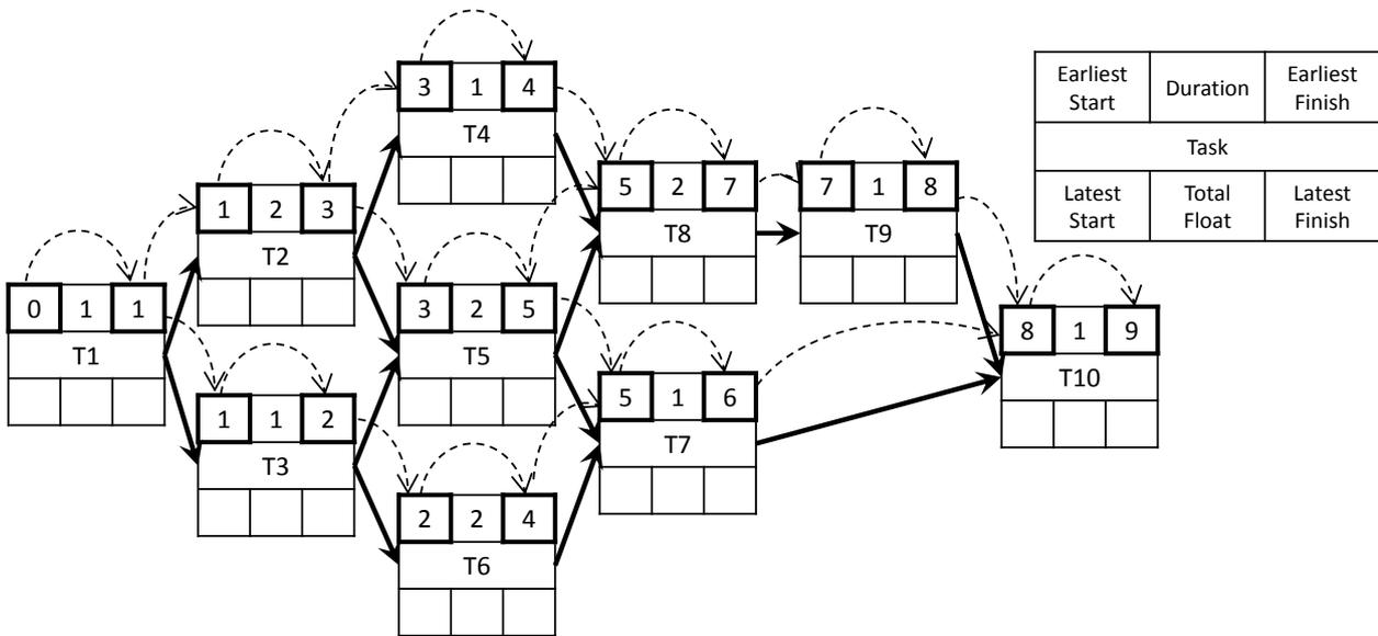
Figure 2-8: Schematic representation of the forward pass for the construction project introduced in Figure 2-1. Determination of the earliest start and finish date of the tasks. Boxes: tasks, arrows: precedence relationships, dashed arrows: steps of the calculation.
