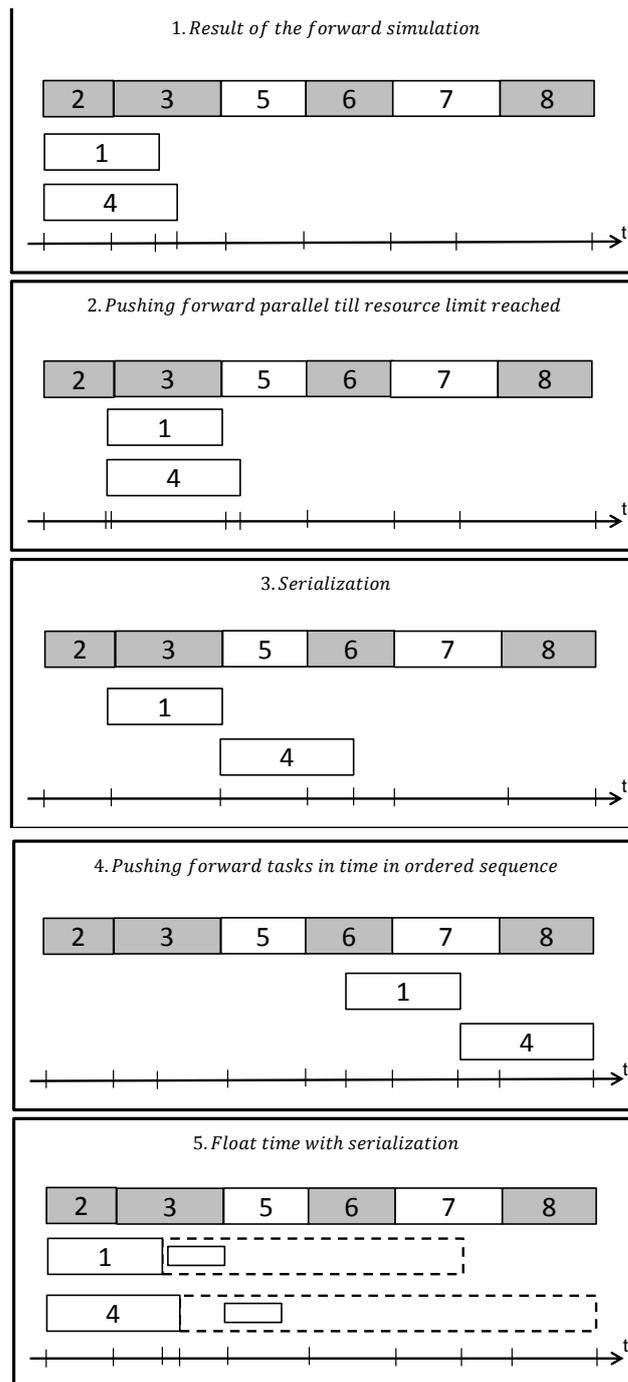
Figure 5-18: The effect of serialization for the determination of float time. (Dashed boxes: float time; boxes in float time: start point and order of serialization)
