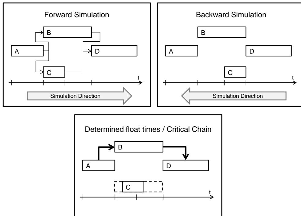
Figure 5-5: Concept of determining total float and critical chain by combining forward (left) and backward simulation (right). (Critical chain: large arrows; float: dashed box)
