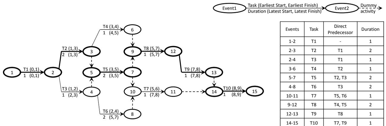
Figure 2-11: Representing the critical path of the construction project introduced in Figure 2-1 on an AOA representation based CPM network. Ellipses: events, thick ellipses: critical events, arrows: tasks, dashed arrows: dummy activities, thick arrows: critical tasks.
