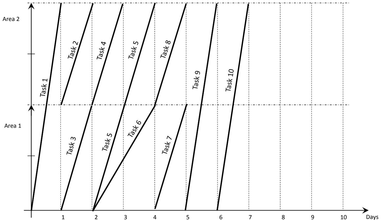
Figure 2-5: Linear schedule representation of the introduced construction project in Figure 2-1. Task 2 and task 8 have been accelerated (duration 1 day) in order to get more parallel execution lines and a more compact schedule.
