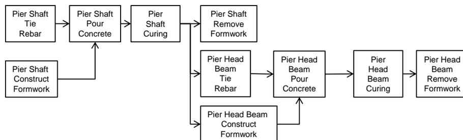
Figure 4-10: Corrected precedence graph of the introduced task sequence in Figure 4-9
