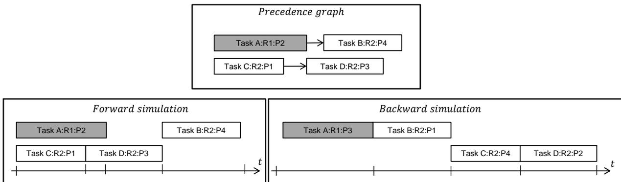
Figure 5-8: Issue with reversed priority settings for the backward simulation: change in the execution order of the tasks (R: resource class, P: priority)
