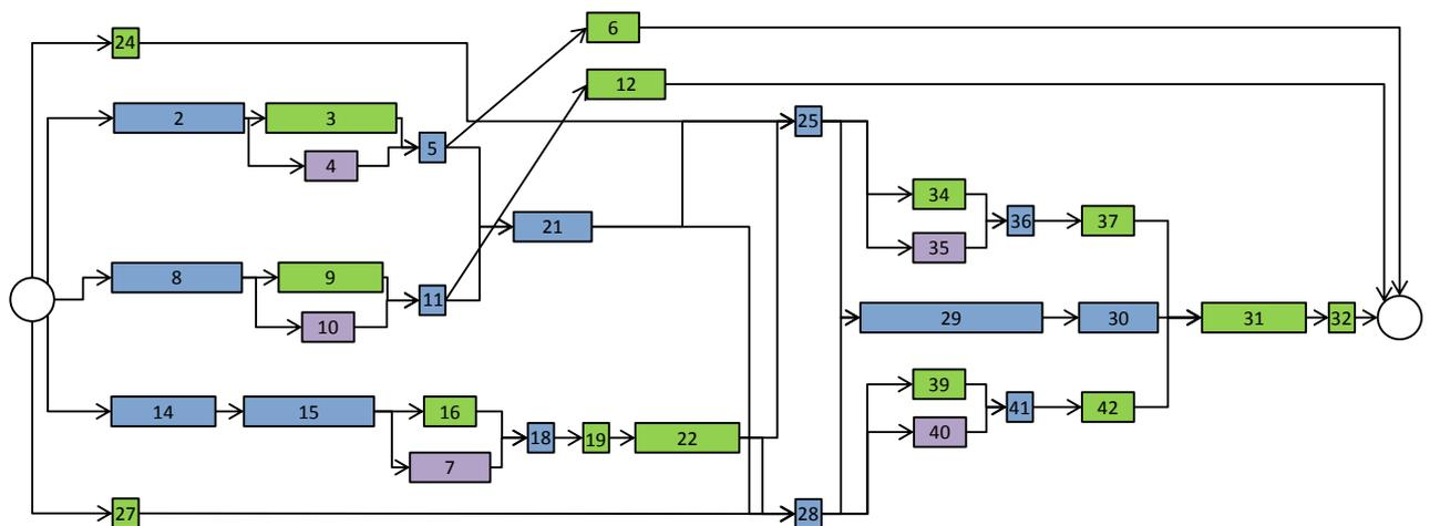
Figure 5-19: Precedence graph of the introduced test case. Colors: resources, such as blue: "concreting", purple: "armouring" and green: "casing".
