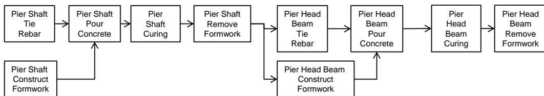
Figure 4-9: Misinterpreted higher-level precedence relationship between the sub-elements of Figure 4-7. The formwork construction and rebar assembly of the pier head beam can already begin when the concrete of the pier shaft is cured.
