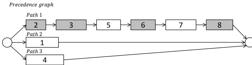
Figure 5-16: An example with large path length differences ( $|Path 1| \gg |Path 2| + |Path 3|$ )
