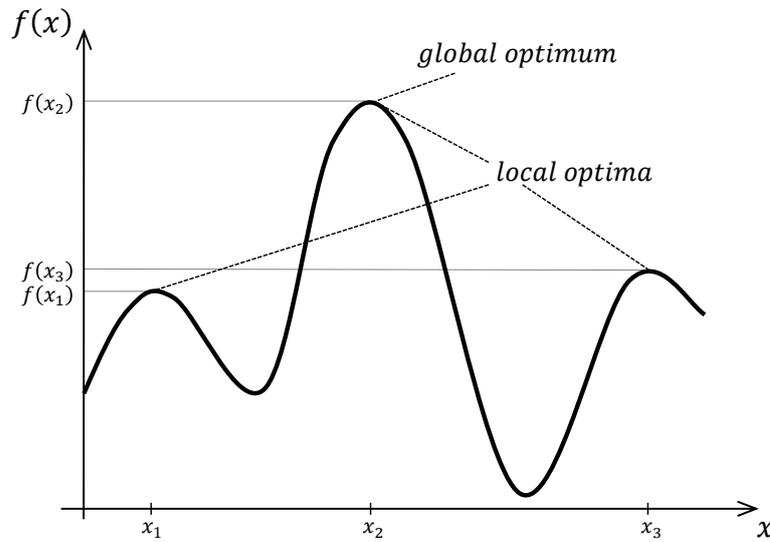
Figure 6-1: Local optima and global optimum of a general continuous single value objective function  $f(x)$  for a maximization problem
