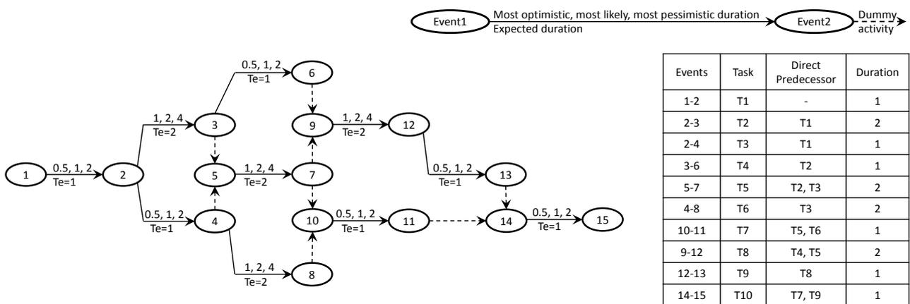
Figure 2-12: AOA-based PERT representation of the introduced construction project in Figure 2-1. On the arrows PERT uses three task duration estimates: the most optimistic, the most likely and the most pessimistic one. Below each arrow is the expected duration of the task.
