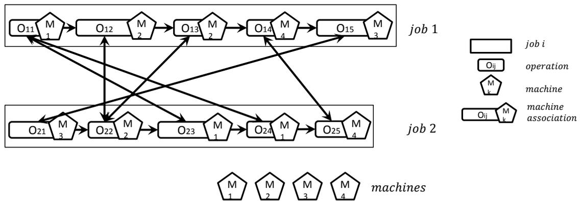
Figure 2-17: Disjunctive graph model of the first two jobs of the introduced job shop problem in Figure 2-16. Simple arrows: conjunctive arcs, double arrows: undirected disjunctive arcs.
