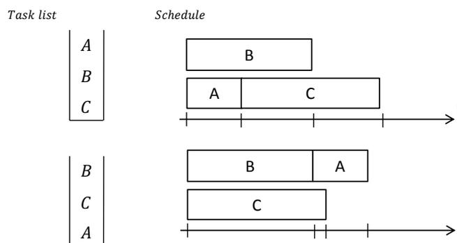
Figure 4-2: Different generated schedules based on the order of tasks within the task list
