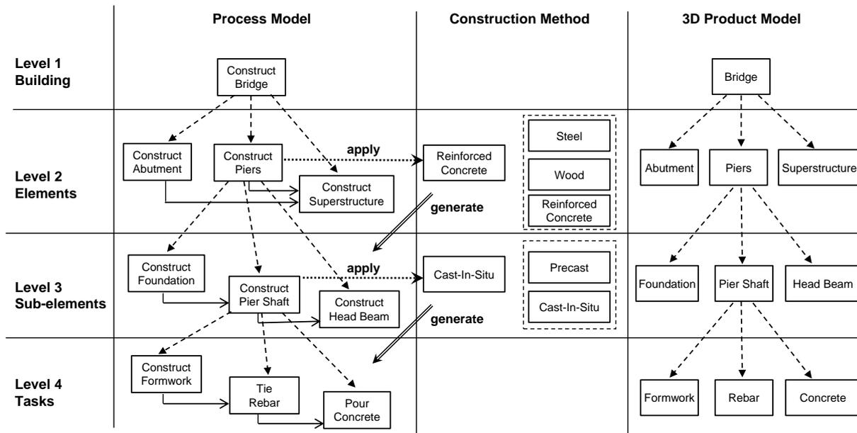
Figure 4-4: Representation of the *levels-of-detail* approach on a simple bridge project. Normal arrows: precedence constraints, dashed arrows: hierarchic decomposition, dotted arrows: construction method selection, double arrows: automatic generation of new components (Wu et al. 2010a).
