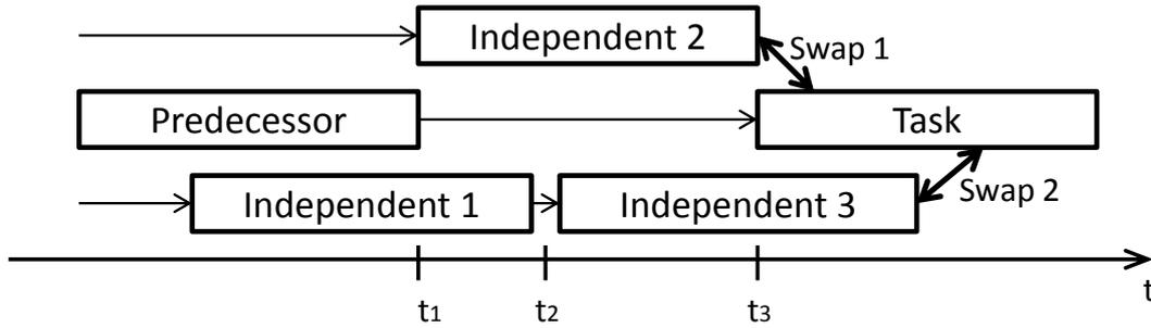
Figure 7-5: Schematic illustration of the reasonable swap determination: the list of possible swaps of independent tasks is restricted by the ones that start between the latest finish date of the task's predecessors (t1) and the task itself (t3). Priorities: Predecessor: 10, Independent 1: 8, Independent 2: 6, Independent 3: 4, Task: 2. Reasonable swaps: Task and Independent 2; Task and Independent 3.
