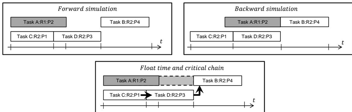
Figure 5-9: Applying the new priorities based on the priority-by-end-date method for the backward simulation. The new priorities are set according to the finish date of the task in the forward simulation. The result is an identical execution sequence of the tasks with the backward simulation, therefore total float and the critical chains are determinable. (Float: dashed gray box, critical chain: large arrows)
