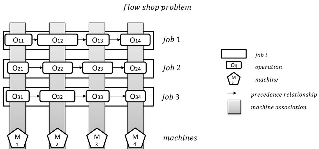
Figure 2-15: Example for a schematic representation of a flow shop problem: the  $m$  operations ( $O_{ij}$ ) of every job are connected as a flow with precedence relationships to each other. Every task is executed on the machine corresponding to the position of the operations in the flow sequence. The task is to find the optimal execution order for the jobs.
