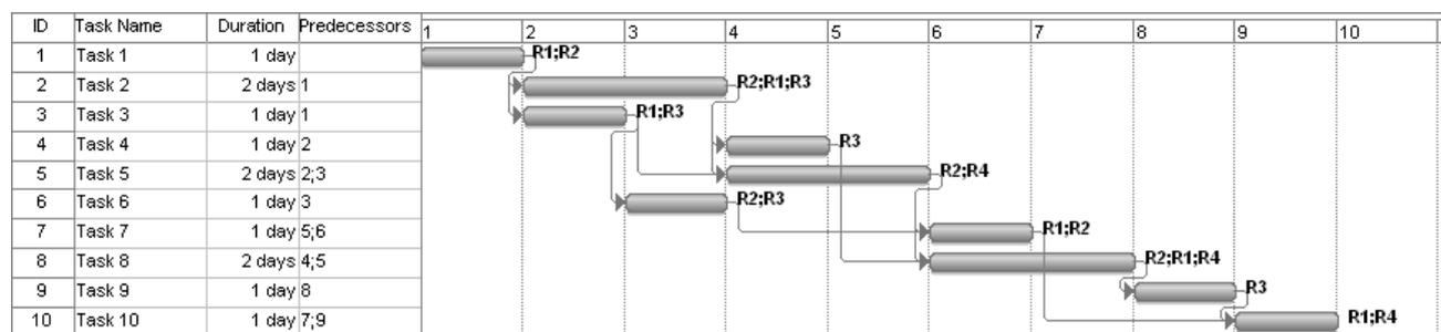
Figure 2-3: Gantt chart representation of the introduced construction project in Figure 2-1. The bars represent the planned execution time interval of a task. Behind the bars the for the tasks execution necessary resources are illustrated. The interrelationships between the tasks are hardly traceable. (MS Project 2007)
