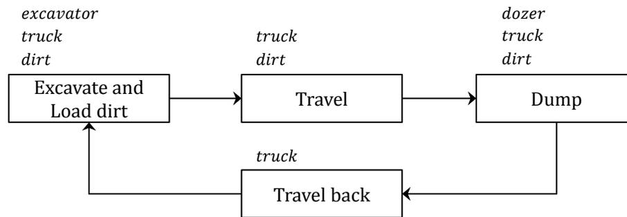
Figure 3-17: ABC representation of the simple earth moving system that has been introduced in Figure 3-13
