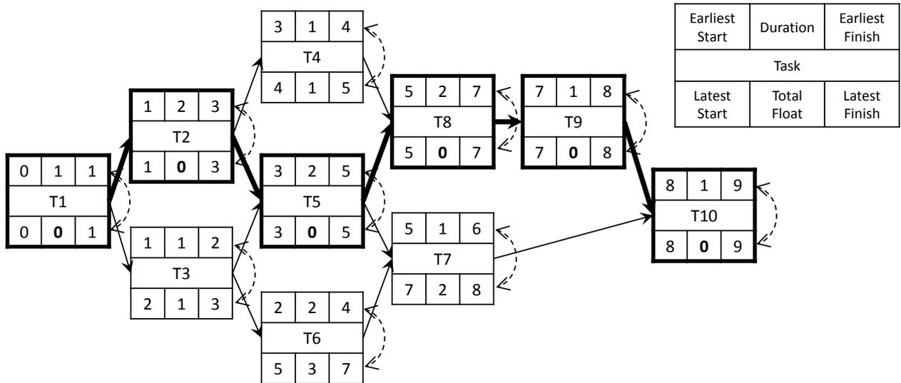
Figure 2-10: Determination of float time and critical path for the construction project introduced in Figure 2-1. Boxes: tasks, arrows: precedence relationships, dashed arrows: steps of the calculation, fat arrows: critical path, fat boxes: critical tasks.
