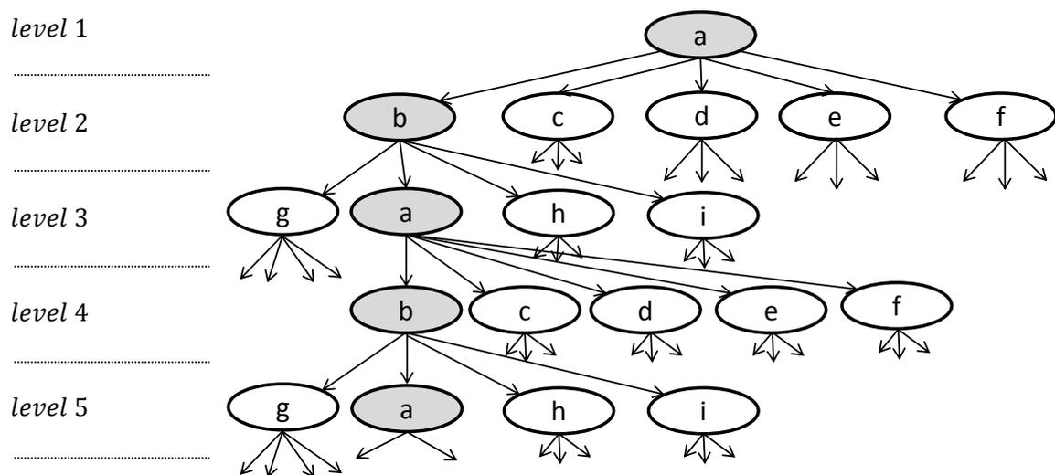
Figure 7-8: The effect of re-swapping: a loop inside the enumeration tree. The child nodes of *node a* and *node b* are determined at every 2<sup>nd</sup> level. The nodes represent a feasible schedule. The re-swapping is marked with gray node-background. To avoid this behavior a tabu search algorithm is applied that forbids to re-swapping of previously swapped priorities.
