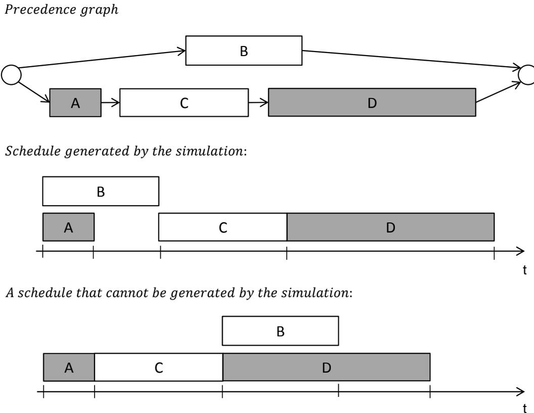
Figure 7-1: Limitation of the constraint-based discrete event simulation: In some cases the complete set of results does not contain the optimal schedule (minimal makespan). White and grey: two resource classes.
