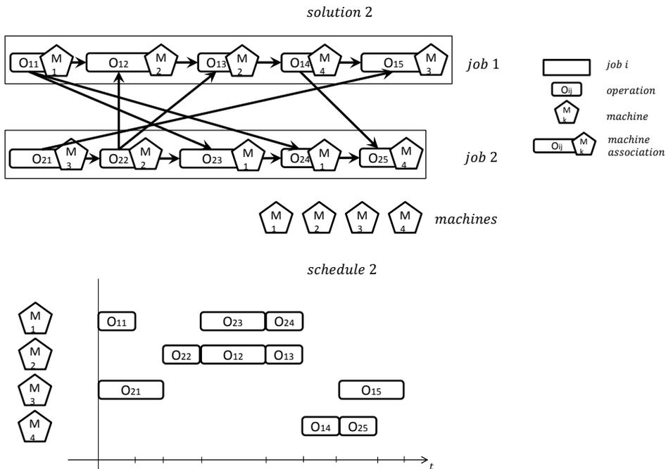
Figure 2-19: Another feasible solution for the introduced disjunctive graph in Figure 2-17. By comparing the resulting feasible schedules of solution 1 and solution 2 it can be seen that schedule 2 is significantly shorter than schedule 1.
