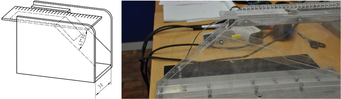
Figure 5.1. Test setup for the characterization of the bending behaviour of uncured prepreg material with conventions (left [110]) and the actual setup (right)
