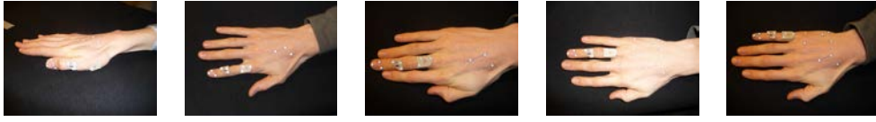
Figure 5.2: Placement of the markers on the fingers for the MoCap experiment. One finger is measured at a time, with the marker sets moved from finger to finger and a constant set of three markers on the back of the hand (Figure 5.2). This is done to facilitate automatic labelling of the markers according to the edge lengths of the triangles that they form.
