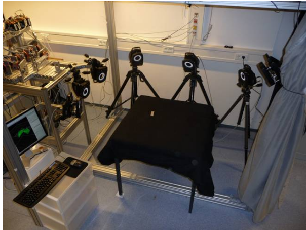
Figure 5.1: The setup of the cameras for the MoCap measurements. The cameras are placed around the workspace, approximately in a semi-circle with a radius of 1 m.
