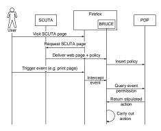
Figure 1: High level sequence diagram of the system
