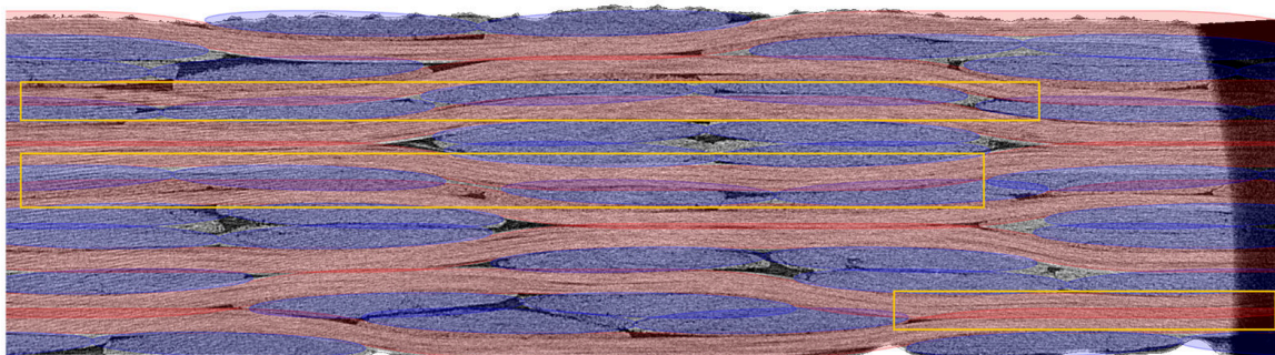
Fig. 5.2: Comparison of yarn geometry of WiseTex and from micro-CT scanning
