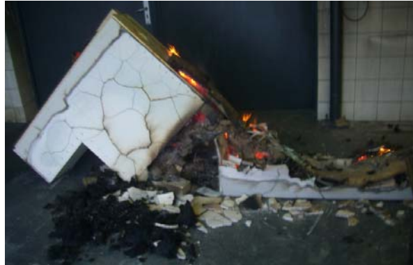
Figure 21 Small-scale fire test with loose wood fibre and gypsum fibre boards in 18 mm (left) and 15 mm (right) after 15 hours of observation
