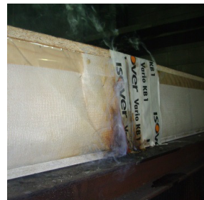
Figure 8: production of smoke as a consequence of glowing combustion in the gap
