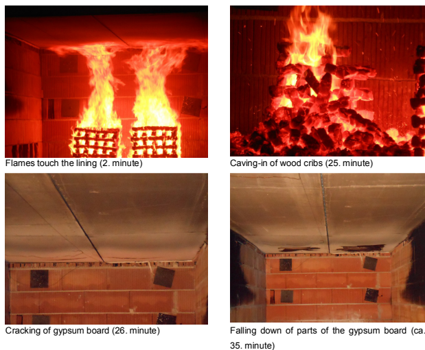
Figure 17: fire progress using the example of test 1
