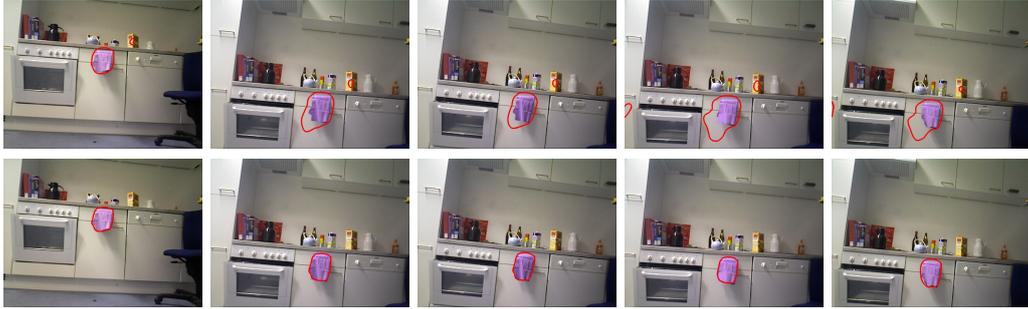
Figure 5.2: Comparison of tracking an object with and without area constraint of a scene captured from a flying quadrocopter. **First row:** Color-only tracking. **Second row:** RGB-D tracking: The surface area is constrained on the absolute dimension via additional information from the depth images.
