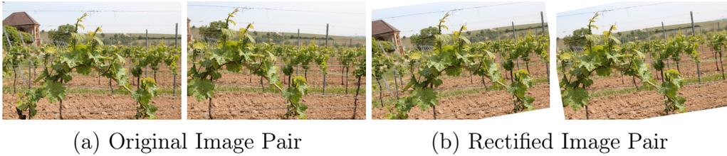
Figure A.1: Example for Image Rectification. In the rectified image pair, epipolar lines are parallel, simplifying subsequent computations of disparities. Rectifications were computed using software of [56] and [99].
