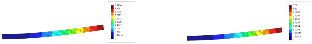
Figure 3.14: Deformation plots of beam bending, Left: Case2; Isotropic strain energy density function and Stretch energy density function, Right: Case3; Istropic strain energy density, Stretch energy density and Bending energy density functions
