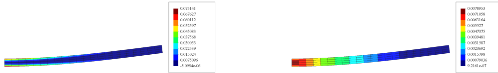
Figure 3.15: Energy distribution plots of beam bending, Left: Stretch energy distribution, Right: Case3; Bending energy distribution
