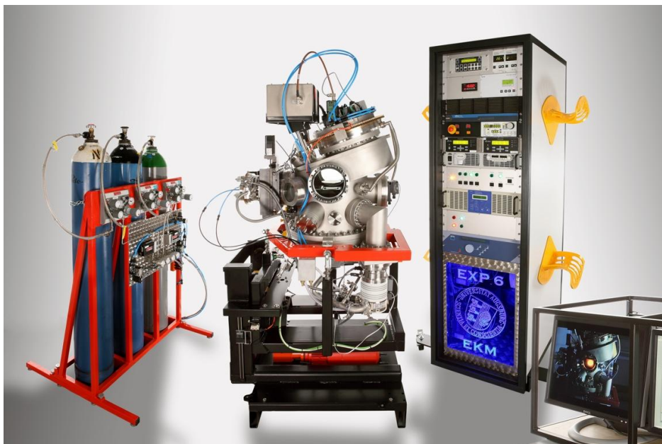
Fig. 3.11: Photo of the sputtering system with the mobile components: the sputtering chamber in the center, the gas rack on the left, and the electronic rack and the computer on the right. (Source: [77])
