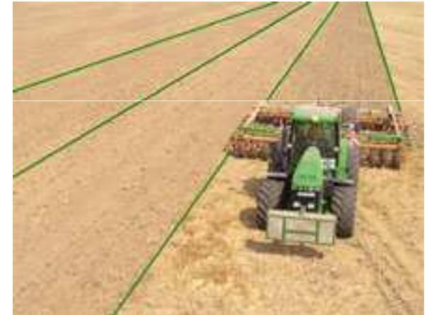
Automatically steers the tractor via hydraulic valve and becomes part of the machine.
