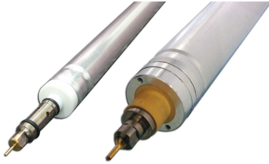
Figure 2.17: Photograph of sMDT (left) and MDT (right) drift tubes.
