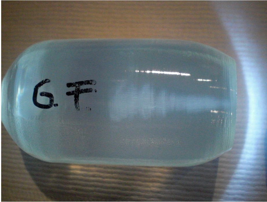
Fig. 3.6: Photograph of the crystal "Georg Friedrich" which shows a high concentration of inclusions (shaded area along the central axis).
