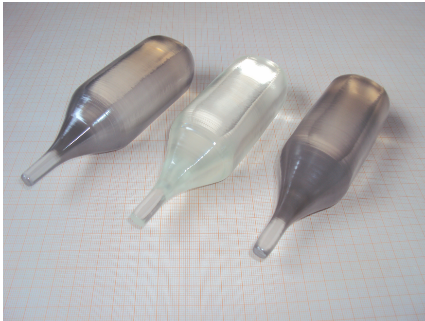
Fig. 2.11: The picture shows the influence of oxygen annealing on the grown crystals. After growth large crystals show a grey coloration due to an oxygen deficiency (left and right crystals). This can be compensated by annealing them in pure oxygen resulting in clear crystals (middle crystal).
