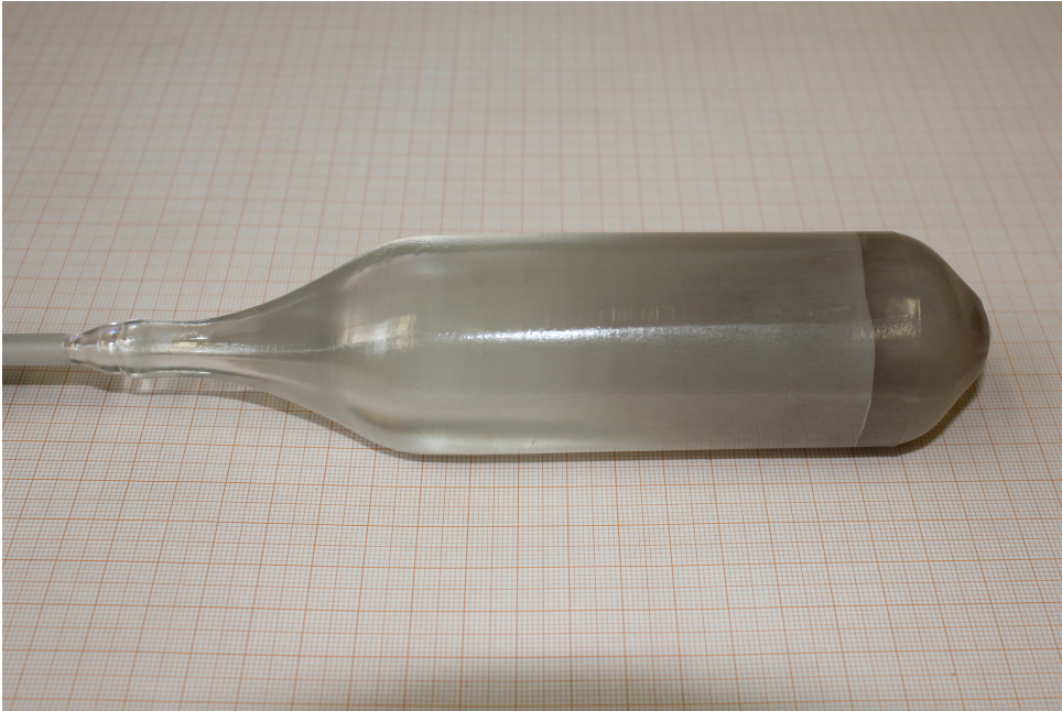
Fig. 2.9: The crystal "Georg" was grown as the 5th crystal without intermittent cleaning of the crucible. The cloudiness that is visible and increasing towards the tail comes from impurities which have accumulated in the melt after each growth.
