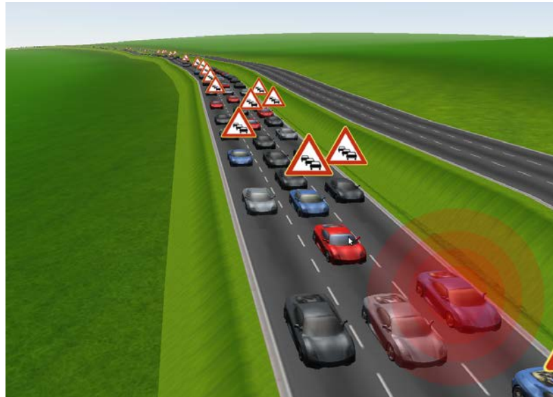
Figure 8-5: Vehicles receiving warnings about a traffic jam; communication shown.
