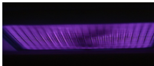
Figure 2.4: Inhomogeneous discharge pattern with welding grid.
