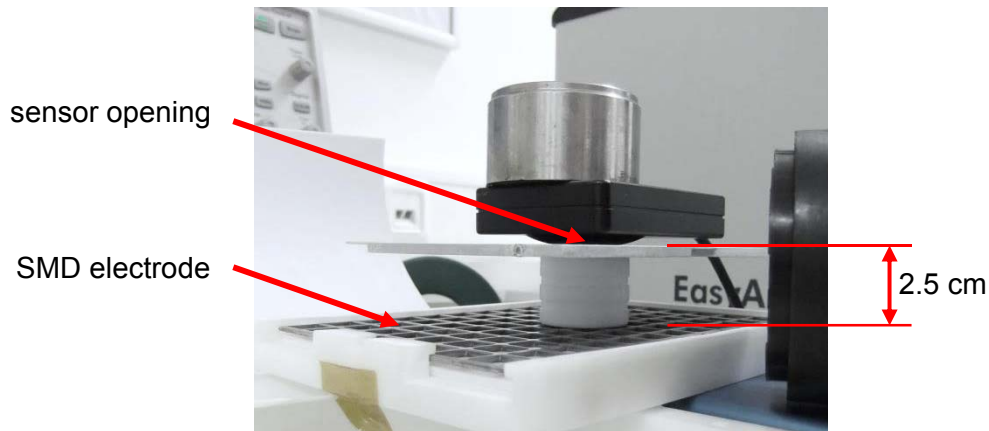
Figure 2.7: UV power measurement set-up.
