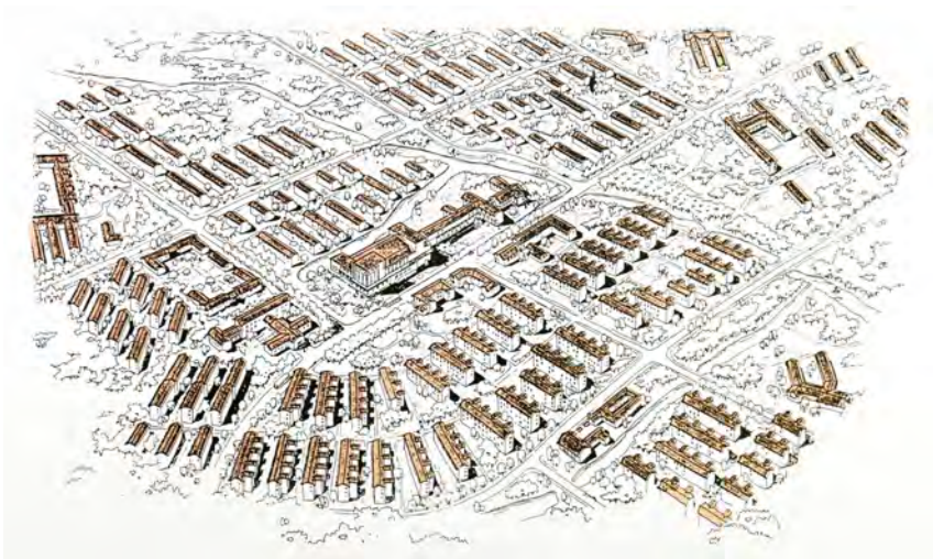
Figure 4.9: An Aerial View of Caoyang New Village (1951-1988). Located in the middle of Putuo District, Caoyang New Village is the first worker village in Shanghai. Started in 1951, the whole housing scheme consists of 9 living quarters and accommodates a population of 107,000 in 32,000 households. The site area is about 180 ha., with a total floor area of 1,697,800 m 2 . From SCC (Shanghai Construction Commission), The Album of Shanghai Housing (Shanghai: Shanghai Scientific and Technological Literature Publishing House, 1998), 81.
