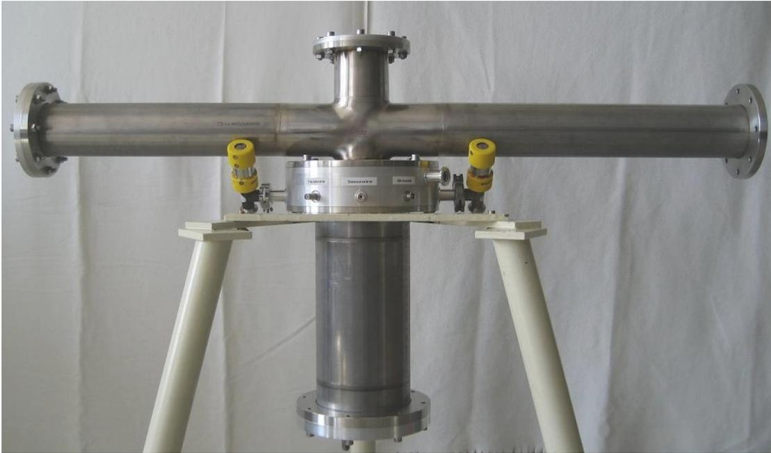
Figure 2.13: *A side view on the experimental setup. The neutron beam enters the setup on the left and propagates horizontally through the cross piece. A target holder is inserted from the top, positioning the foils in the neutron beam. The multi-wire chamber is situated between the two yellow gas in- and outlet valves, 9 cm beneath the neutron beam. The lower part houses the scintillator and the photomultiplier, which looks towards the target position.*
