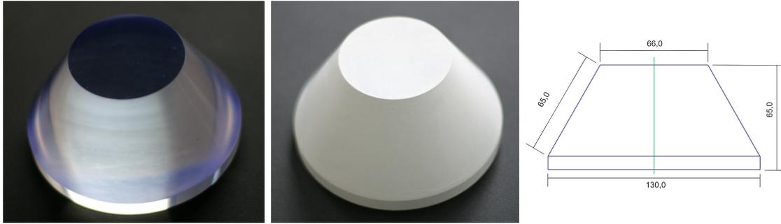
Figure 2.8: *The plastic scintillator used. On the left, the original plastic scintillator is seen, in the middle the scintillator is thinly covered with reflective paint. The geometry of a truncated cone (right, values in [mm]) assures that electrons from the target entering the scintillator on the top deposit their whole energy and do not leave the detector at the sides.*
