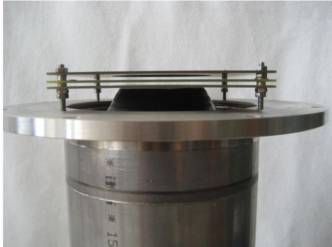
Figure 2.12: *The spectroscopic module (see also fig. 2.9) is inserted into the detector steel pot and the MWC is positioned 1 mm above the plastic scintillator. One can recognise the three boards of the MWC with a total height of the chamber of 10 mm. This combined module is then mounted to the cross piece as indicated in figs. (2.6), (2.7) and (2.13).*
