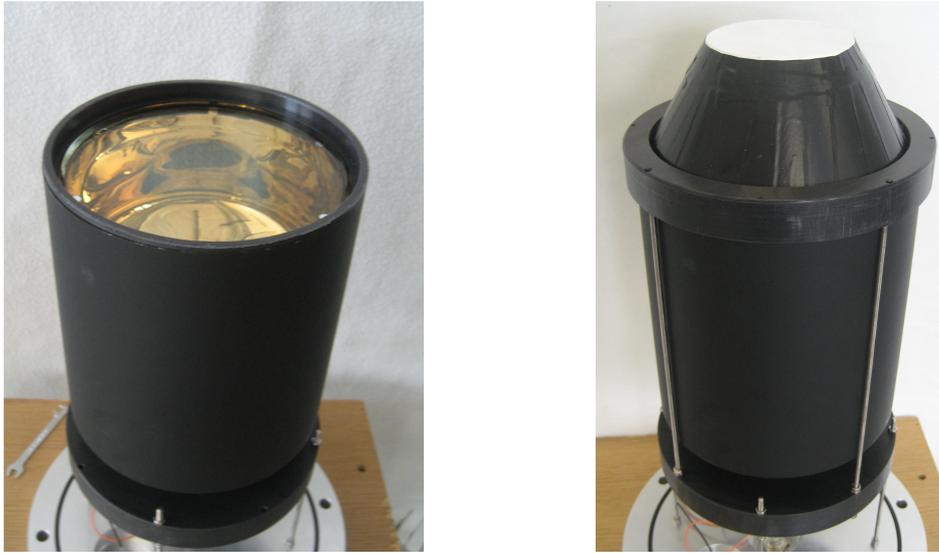
Figure 2.9: *The spectroscopic module consists of the plastic scintillator, partly covered by reflective paint and wrapped in black tape, and the photomultiplier, shielded from magnetic fields by the Mu-metal mantle.*
