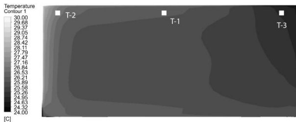
Figure 8b: Temperature difference in the sun space - CFD simulation
