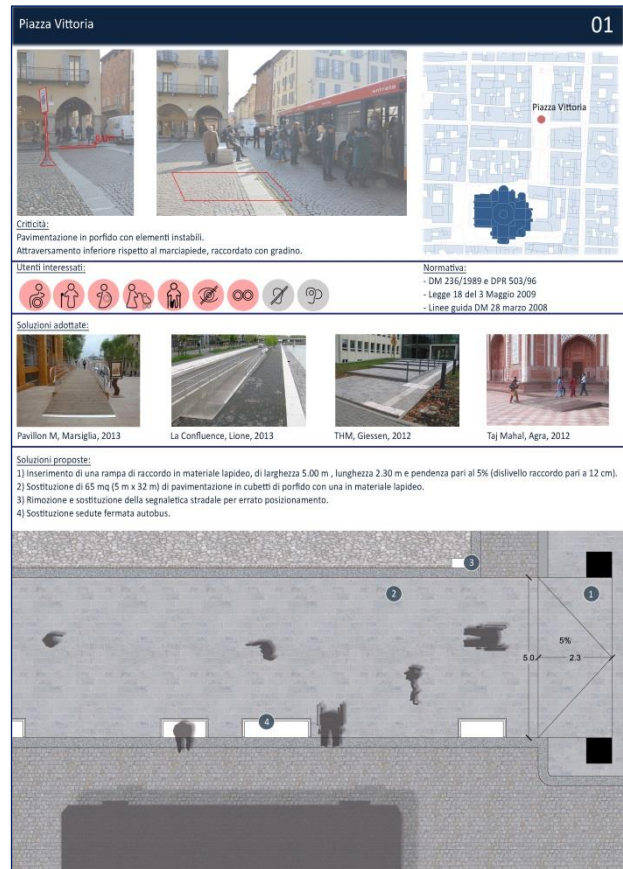
Figure 4: Chart for the proposal of architectural solutions for Piazza della Vittoria. The main problem identified in this case is the difference in level between the porches and the square. The solutions consist of the project of a ramp, a new paving with the same material (stone slabs) and a new urban furniture near the bus stop. These solutions are appropriate to people with mobility impairments and to people with sensory impairments.
