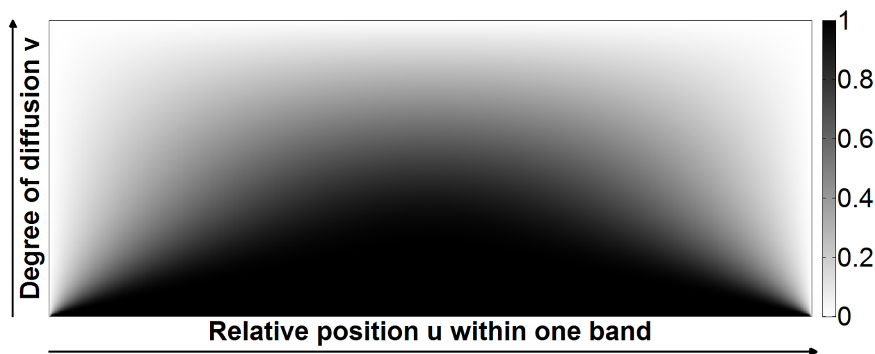
Figure 5.26: The diffusion texture T . Diffusion values from 0 to 1 are mapped to a grayscale color map. The x-axis represents the relative position u of a point between two band boundaries. The y-axis represents the degree of diffusion v .
