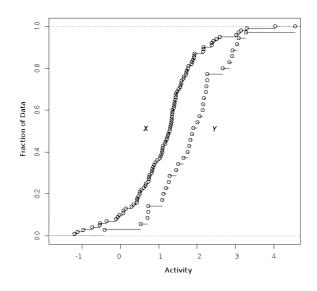
FIGURE 3.4: Comparison of the cumulative activity distributions of two (hypothetic) sets of activity values X and Y with sizes 100 and 35, respectively. The mean value of X is 1.0, the mean value of Y is 2.0. It is highly unlikely (KS test gives p = 0.0001319) that X and Y have been drawn from the same data source.
