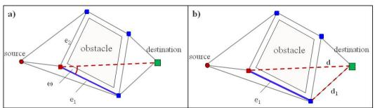
Fig. 3 a) angle derivation  $\omega$  of edge e<sub>1</sub> b) relative distance enhancement of edge e<sub>1</sub>: d<sub>1</sub>/d
