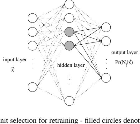
**Fig. 2.** Unit selection for retraining - filled circles denote selected nodes, thick lines indicate weights to be retrained
