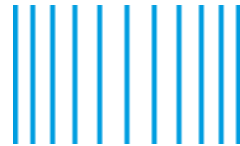
Figure 7.24: Printed phantom consisting of 11 vertical lines of a thickness of 0.1 mm and a distance of 0.9 mm in the center. The distance towards the edges was reduced by 0.1 mm for each new line down to 0.5 mm. The outer dimensions of the phantom measures 92 \times 56 \text{ mm}^2 .
