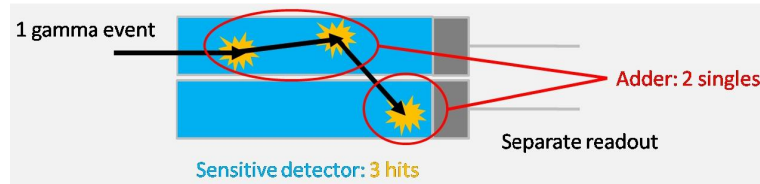
Figure 4.3: Principe of the adder and readout module [30].
