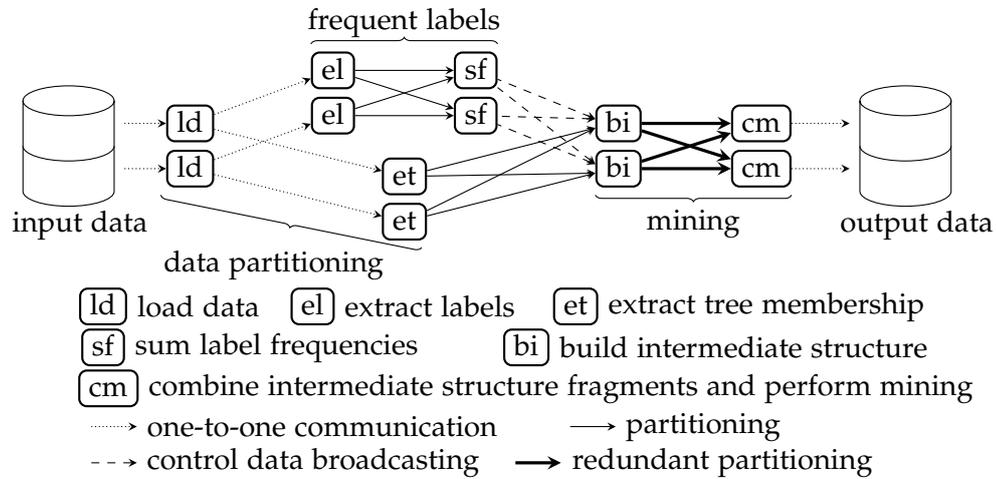
Figure 2.4: Distributed Tree Mining Workflow
