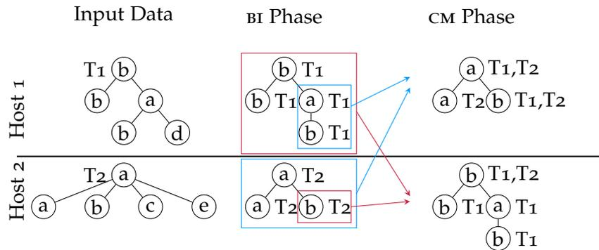
Figure 2.5: Distributed Path Join
