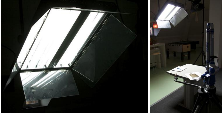
Figure 2.7: The daylight panel mounted above the target. The panel was adjusted by switching on/off five independent fluorescent tubes.
