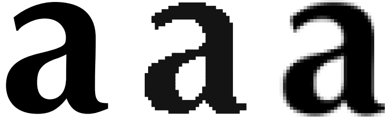
Figure B.1: Example for interpolation. From left: vector image of the letter “a”, nearest-neighbour and bilinear interpolation to a resolution of (40 \times 43) .
