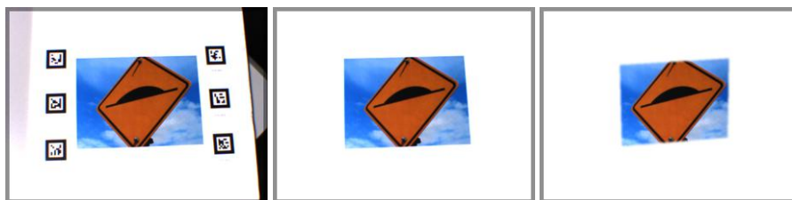
Figure 2.17: Post-processing. From left : captured image, undistorted image without background, final image with randomized borders.
