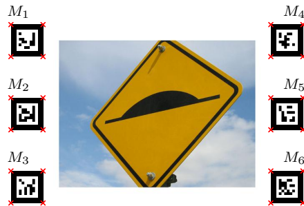
Figure 2.11: A target used for evaluation with six fiducial markers M_1 \dots M_6 around it. The outer corners \bar{\mathbf{x}}_{m,i} of the markers M_m , highlighted with red crosses, are used for the refinement of {}^{base}\mathbf{T}_{target} and for synchronization.
