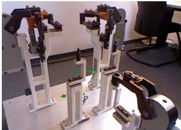
Figure 4.13: Maintenance instructions can be better understood when their occlusions are handled correctly as done for the lower of the two wrenches.
