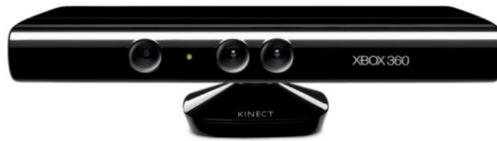
Figure 4.1: RGB-D camera Microsoft Kinect. From left: IR projector, RGB camera and IR camera. © Microsoft
