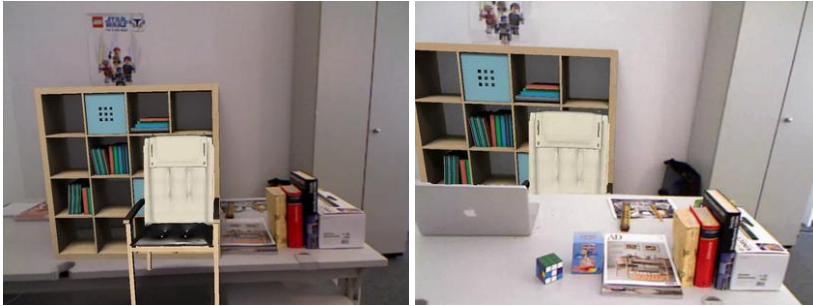
Figure 4.11: AR-based virtual furniture trial: correctly handling the occlusion thanks to the proposed parallel tracking and meshing of the environment makes the AR visualization much more realistic. While the camera moves, the camera motion is estimated and the environment model is updated.
