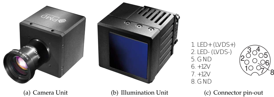
Figure 6.14.: Camera and illumination units. Pin-out of the cable between
