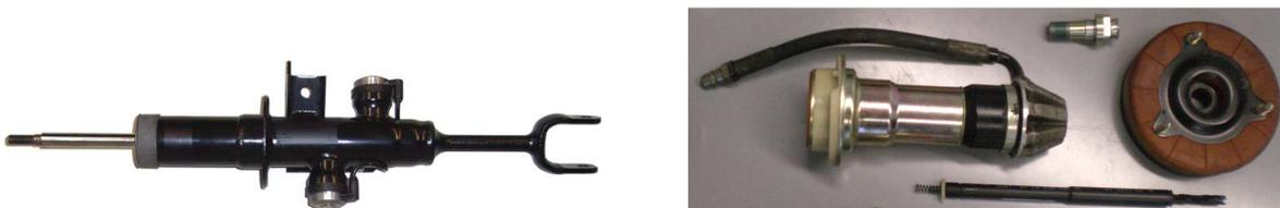
Figure 2: Continuously variable damper (*BMW 7 series*) and components from the hydraulic *Mercedes Benz - Active Body Control* suspension system.
