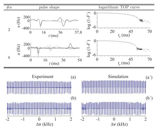
Table 6.6: Numerical results for a more generally-coupled four-spin systems with coupling ratios  $k_1 = 2.38 \approx J_{12}/J_{23}$  and  $k_2 = 0.94 \approx J_{34}/J_{23}$  (i.e.  $J_{12} = 46$  Hz,  $J_{23} = 19.3$  Hz, and  $J_{34} = 18.1$  Hz) as well as additional couplings  $J_{13} = 4.1$  Hz and  $J_{24} = 2$  Hz. Compare to Table 6.3.
