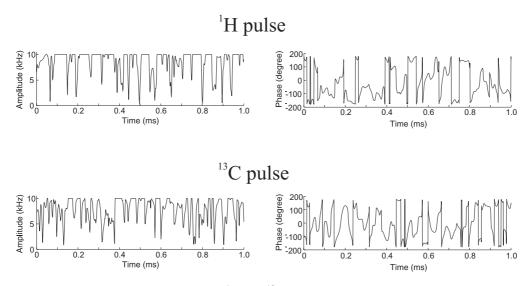
Figure 7.9: The amplitude and phase of  ${}^{1}$ H and  ${}^{13}$ C pulses optimized simultaneously are plotted as a function of the pulse duration. All are 1 ms long with a maximum amplitude of 10 kHz.
