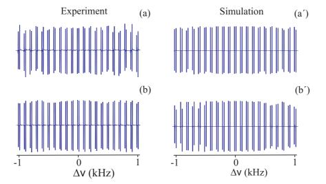
Figure 6.9: (Color online) We compare for a three-spin system the offset  $(\Delta v)$  profile for  $\pm 1$  kHz of the anti-phase signal (see text) resulting from a conventional pulse sequence  $(t_p = 11.4 \text{ ms})$  in the case of experiment (see (a)) and simulation (see (a') with broadband versions of the analytic pulses  $(t_p = 9.8 \text{ ms}, \text{see (b) and (b')})$  for the case of coupling ratio k = 1 of three spins.
