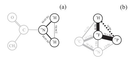
Figure 6.3: The schematic coupling topologies of (a) ethanamide and (b) diethyl-(dimethylcarbonyl)fluoromethylphosphonate (see [201, 202]) result in experimental three-spin systems with coupling ratios (a) k = 1 = 88.05/88.05 and (b)  $k = 1.59 \approx 73.1/46$ . Larger couplings are shown as solid-black lines, and smaller couplings are shown as dashed-black lines. Decoupled spins are given in gray color.
