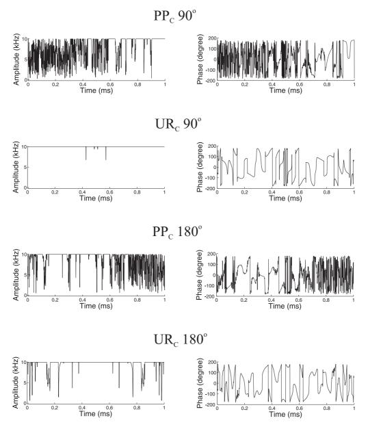
Figure 7.18: The amplitude and phase of  ${}^{13}C$  pulses are plotted as a function of the pulse duration. All are 1 ms long with a maximum amplitude of 10 kHz.
