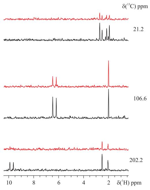
Figure 7.8: (Color online) Traces through cross signals at 21.2, 106.6 and 202.2 ppm are compared for conventional-HMBC (red, top) and Fanta4-HMBC (black, bottom) (Fig. 7.7). The Fanta4-HMBC sequence gives improved S/N ratio compared to the conventional-HMBC sequence.
