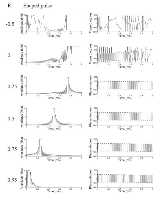
Figure 3.4: The RF amplitude and Phase are plotted as a function of time for a series of 1 ms pulses designed using different values of R and with  $RF_{lim}$  of 10 kHz to excite a bandwidth of  $\Delta \nu = 50$  kHz.
