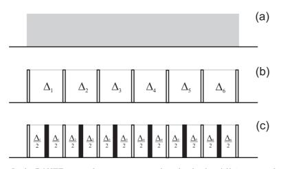
**Figure 6.8:** In the DANTE approach an on-resonance shaped pulse (see (a)) is converted to a series of short hard pulses and delays  $\Delta_i$  (see (b)). Then, the pulse can be converted to a broadband pulse by inserting a refocusing element (i.e.  $\pi$ -pulse) represented by solid bars between two hard pulses (see (c)).
