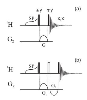
**Figure 5.5:** (a) Phase-cycled sequence consisting of excitation by selective pulse (SP), hard  $90^{\circ}$  pulse, gradient pulse, hard  $90^{\circ}$  pulse, and acquisition. The sequence is designed to eliminate residual *y*-magnetization produced either by standard selective pulses in the presence of RF inhomogeneity or produced by design in the case of RC-SEBOP (b) a single-acquisition sequence designed as an alternative to (a).
