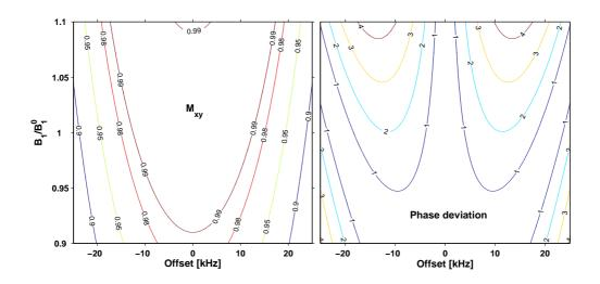
Figure 3.1: (Color online) Performance of a 16.7  $\mu$ s hard pulse, peak RF amplitude = 15 kHz. Transverse magnetization  $M_{xy}$  (left panel) and absolute value of the phase deviation from linearity (right panel) are plotted as functions of resonance offset and RF miscalibration/inhomogeneity  $B_1/B_1^{\circ}$ .  $B_1$  is the variable RF amplitude and  $B_1^{\circ}$  is the nominal RF amplitude.
