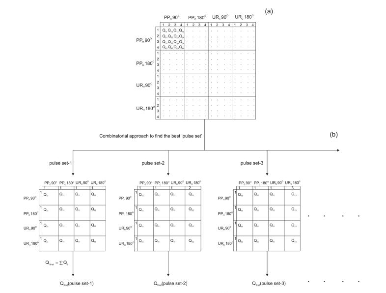
Figure 7.15: It depicts the combinatorial approach to select the best set of pulses. Figure (a) list the selected pulses with fidelity  $Q_{ij}$ , where i and i are indices for the pulse combination. Figure (b) shows the possible sets of pulses and calculation of the combined fidelity  $Q_{final}$  for each pulse set.
