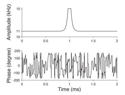
**Figure 4.2:** The amplitude and phase of  $180^{\circ}_{UR}$  pulse 4 from Table 1 obtained using algorithm  $A_{S,T}$ . A conservative limit of 11 kHz for the peak RF applied for 2 ms is relaxed to allow a safe peak of 15 kHz for 60  $\mu$ s. The pulse is amplitude-symmetric and phase-antisymmetric in time, incorporating the symmetry of the construction procedure from Ref. [41].
