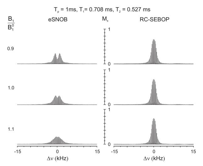
Figure 5.7: Same as Fig. 5.6, but applied to a faster-relaxing sample with  $T_1 = 708 \ \mu s$ ,  $T_2 = 527 \ \mu s$ . Although RC-SEBOP was optimized for  $T_1 = T_2 = T_p = 1 \ ms$ , it provides excellent resistance to relaxation for much shorter values, preserving 75% of the initial magnetization on-resonance for the case  $B_1/B_1^0 = 1$ .
