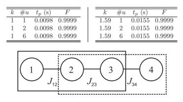
Figure 6.4: A linear four-spin chain has only direct couplings  $J_{12}$ ,  $J_{23}$ , and  $J_{34}$  between neighboring spins. We split the corresponding four-spin chain control problem into two subproblems for three-spin chains.
