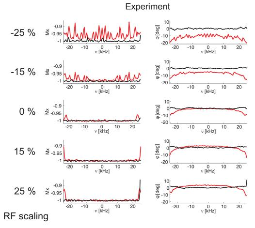
**Figure 4.6:** (Color online) Experimental measurements of the inversion profile (left) and phase deviation (right) corresponding to the simulations in Fig. 4.5, showing excellent agreement between the experimental and theoretical performance of the pulses.
