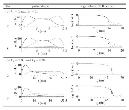
and eight RF controls (see Table 6.3) indicate that we do not gain a higher fidelity or a shorter duration from using more than the two controls (Table 6.4). This is consistent with the analytic results, but the numerically-optimized pulses appear to be a little shorter than the analytical ones (cp. Fig. 6.5).
