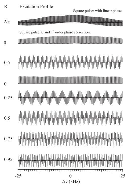
Figure 3.5: Excitation profile of ICEBERG pulses with different R (Fig. 3.4) compared with hard pulse ( $T_p = 16.7 \ \mu s$ ).
