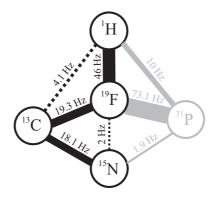
**Figure 6.6:** The topology of the <sup>13</sup>CO<sub>1</sub><sup>15</sup>N-diethyl(dimethylcarbonyl)fluoromethylphosphonate (see [201, 202]) results in coupling ratios  $k_1 = 2.38$  and  $k_2 = 0.94$ . Compare to Fig. 6.3.
