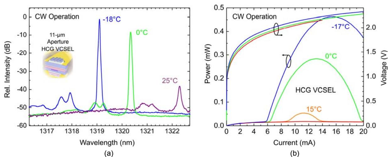
**Fig. 2.** CW performance of the HCG long-wavelength VCSEL. Highly resolved single-mode spectra (a) with no visible polarization mode. Spectra are presented up to 25°C. The tuning coefficient is 0.07 nm/K. The *LIV*-performance (b) shows CW-operation at room temperature and cooled CW-powers in excess of 0.4 mW.
