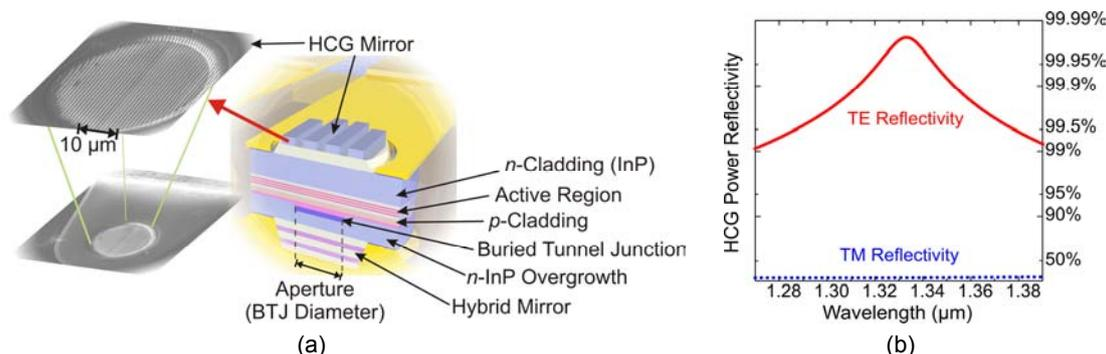
**Fig. 1.** (a) Schematic figure of the cross section of the investigated HCG long-wavelength VCSEL. A scanning electron microscope (SEM) image of the processed device as inset. (b) Simulated HCG reflectivity as deployed on the VCSEL structure. The reflectivity for TE-polarized light is very high over a wide range, whereas the other polarization mode is strongly suppressed.
