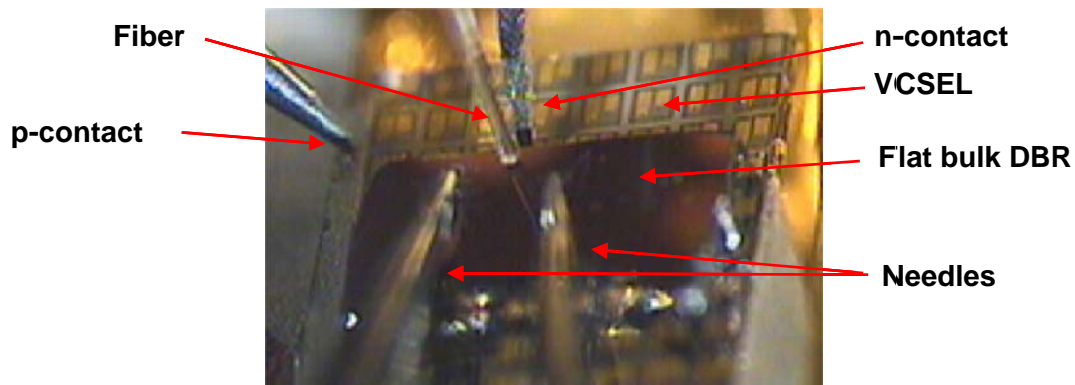
Fig. 8: The tuning of the laser wavelength by the use of a plane bulk dielectric DBR.
