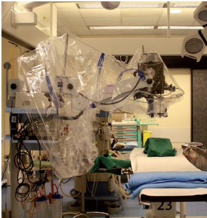
Figure 3-2. Picture of the developed multispectral intra-operative system during measurements inside the operating room. Specialized microscope drapes are used for sterilization, while the small form factor of the setup minimally intervenes in the surgical field.
