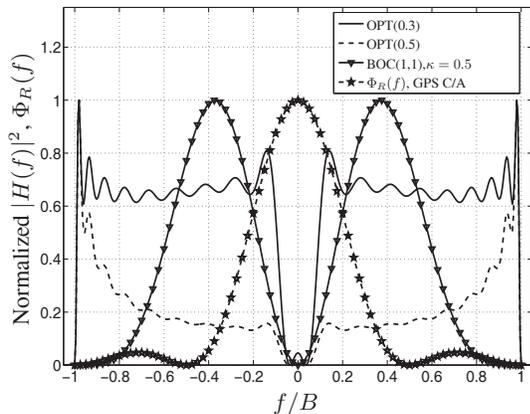
**Fig. 2.** Normalized  $|H(f)|^2$  and  $\Phi_R(f)$ , GPS C/A.
