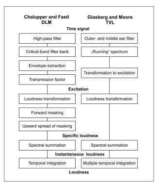
Figure 1. Schematic structure of the loudness models [20] (DLM, left) and [38] (TVL, right).
