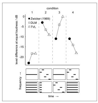
Figure 8. Level differences between test and reference signals at equal loudness for four experimental conditions. Filled circles indicate data of Zwicker [46], open squares and triangles represent predictions of the DLM and the TVL, respectively. The pictograms below show the spectro-temporal pattern of the test (lower row) and reference (upper row) stimuli for each condition.
