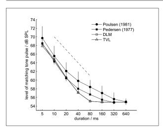
Figure 3. Sound pressure level at equal loudness of 1-kHz tone bursts as a function of burst duration measured by Poulsen [26, filled circles] and in an international round Robin test [39, filled squares]. Error bars represent 95%-confidence intervals of the data of Poulsen [26]. Predictions by the DLM (squares) and the TVL (triangles) are shown with open symbols. The dashed line indicates -3 dB per doubling of duration.
