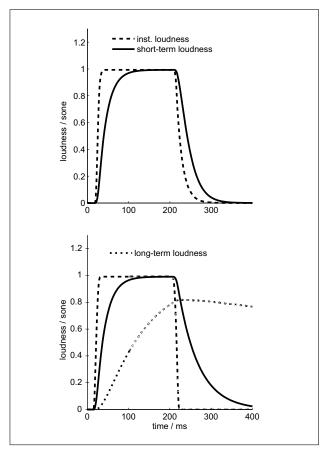
Figure 2. Predicted loudness in response to a 1-kHz tone burst with a level 40 dB SPL and a duration of 200 ms obtained with the DLM (top) and the TVL (bottom). Both panels show the instantaneous loudness (dashed line) and short-term loudness (solid line). For the TVL, the dotted line additionally indicates the predicted long-term loudness.
