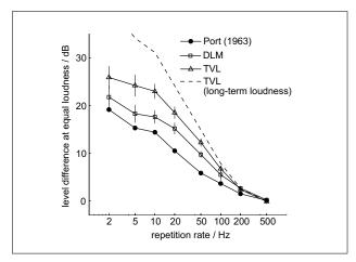
Figure 4. Level difference between repeated 2-ms bursts of narrowband noise and an equally loud continuous noise as a function of repetition rate. Filled circles show the data measured by Port [23], open squares and triangles represent the predictions of the DLM and the TVL, respectively. Error bars for the simulations represent standard deviations over 10 simulations.
