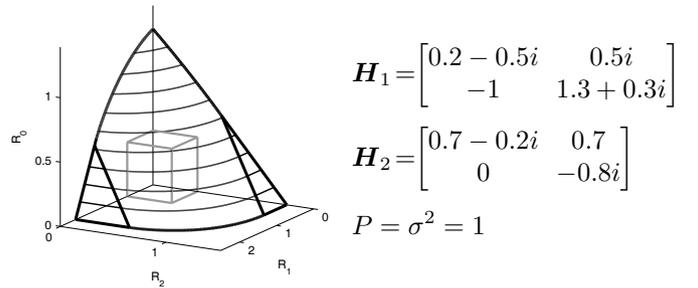
Fig. 2. Capacity region of the MIMO Gaussian BBC with common messages (black) and a comparable TDMA approach (gray) with  $N_R = N_1 = N_2 = 2$ .
