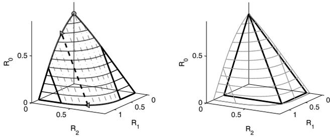
(a) Capacity region of the MISO Gaussian BBC with common messages (b) Achievable rate region for the XOR coding approach (black)
