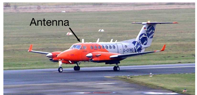
Fig. 5. Beechcraft King Air 350 airplane. The location of the antenna is shown by the arrow. The antenna follows the 743 ARINC configuration.
