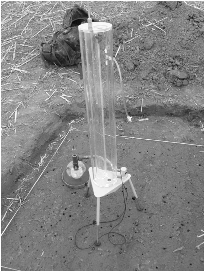
**Figure 1-5: Hood infiltrometer on a macroporous soil in the Weiherbach catchment. Soil hydraulic conductivity was measured for different water tensions, and macropores were mapped.**
