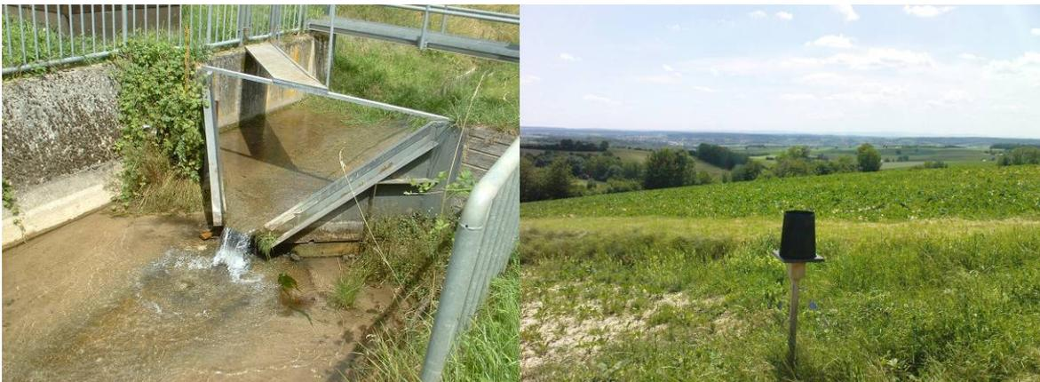
**Figure 2-5: The gauge Menzingen (left), and a Davis tipping bucket (right) on the eastern catchment slopes.**
