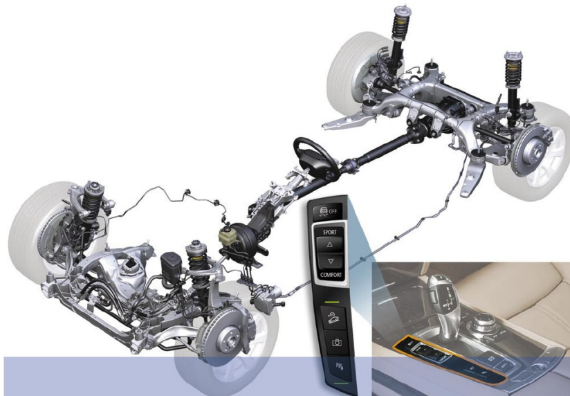
Figure 1.1: Mechatronic suspension system of BMW 7 series (model year 2009) [160]. Image is reproduced with kind permission of BMW AG .
