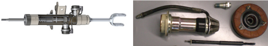
Figure 7.1: Continuously variable damper ( BMW 7 series , see also [1]) and actuator components from the hydraulic Mercedes Benz - Active Body Control suspension system. The left image is courtesy of ZF Friedrichshafen AG and is reproduced with kind permission.
