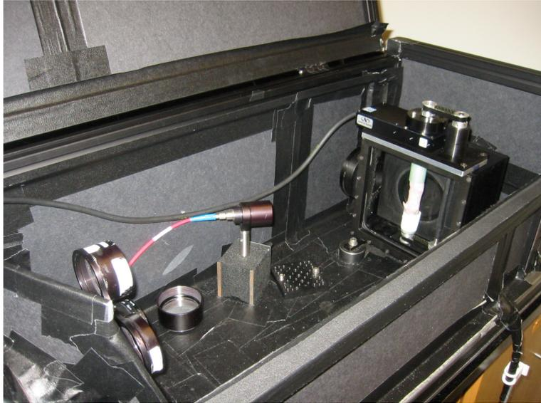
Figure 1.14: Photograph of a FMT system built in 2005 at CMIR, Boston, USA.
