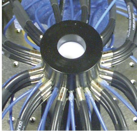
Figure 4.3: First generation FMT setup developed at CMIR utilizing fibers to deliver and collect photons. Reprinted by permission from Macmillan Publishers Ltd: *Nature Medicine* [14], copyright 2003.
