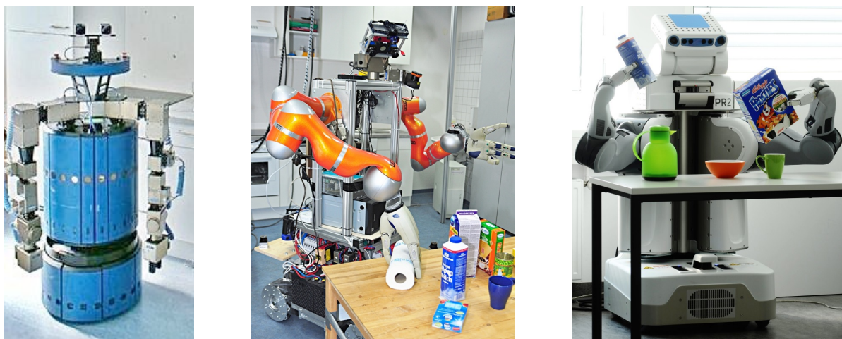
FIGURE 1.3 Left: B21r mobile robot with Powercube arms. Center: TUM-Rosie. A Kuka-based mobile manipulation platform. Right: PR2 manipulating milk and Frosties.
