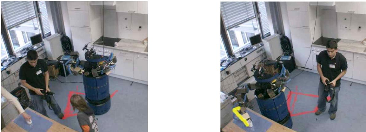
FIGURE 1.1 A reach and grasp trajectory performed by the B21r TUM kitchen assistant during a public demonstration. Left: Robot navigates to table so that the cup is well in reach. Right: Arm reaches for cup. Note that the operator is holding a camera, not a remote control.
