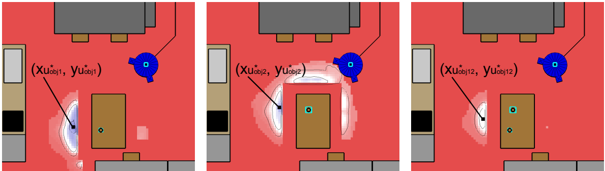
FIGURE 2.4 Left: ARPLACE utility distribution for grasping obj_1 . (x_{u_{obj_1}^*}, y_{u_{obj_1}^*}) is the grid cell with maximum grasp utility for grasping obj_1 . Center: ARPLACE utility distribution for grasping obj_2 . Right: ARPLACE utility distribution for grasping obj_1 with the right hand and obj_2 with the left hand. Blue indicates high grasp utility, white and red successively lower utility.
