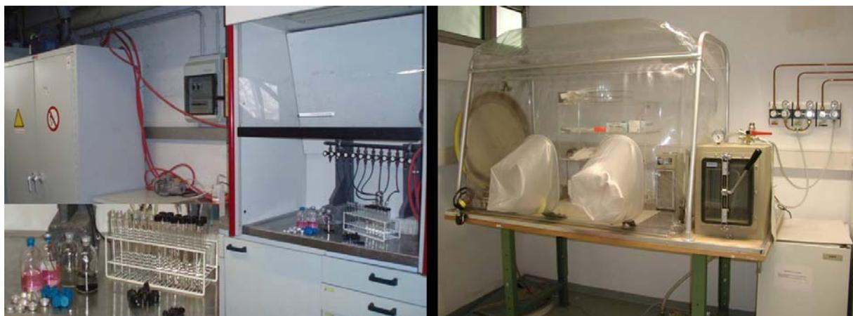
**Fig. 2-1.** Gas station (left) and Anaerobic chamber (right)
