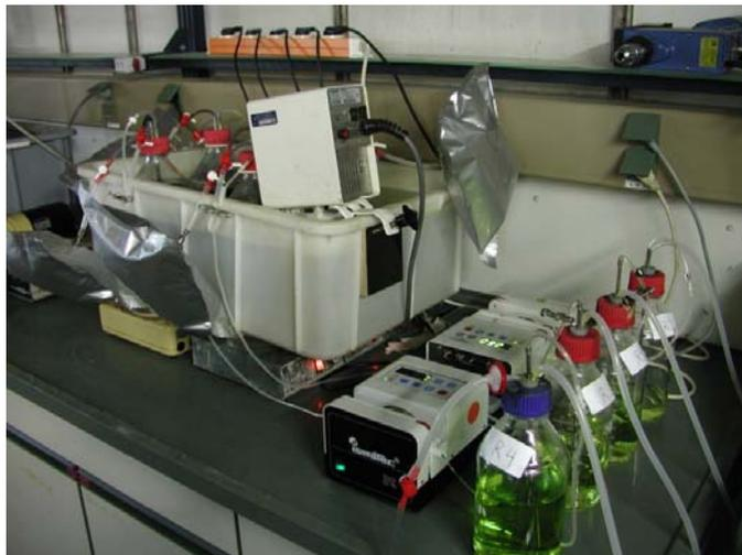
**Fig. 2-2.** Semi-continuous stirred tank reactor (A) configuration, (B) photograph
