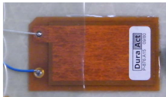
Figure 5.30.: Piezoelectric patch-type actuator
