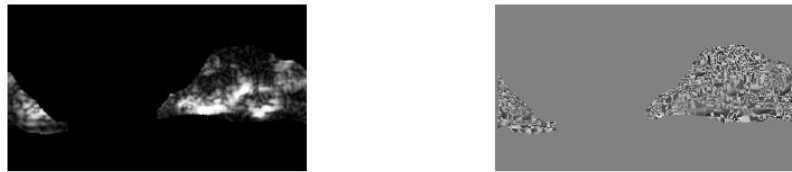
Figure 5.47.: Illustration of Hu feature f_6 : Plaque Area in Polar Coordinates (left) and f_6 (right).
