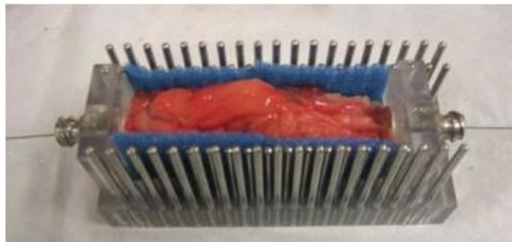
Figure 4.5.: Tissue cage fixture: The artery is fixed in the cage and an automatic pullback is performed in saline and human blood. The histology sections are taken at every 2 mm using side rods after the artery was fixed by formaldehyde[38].
