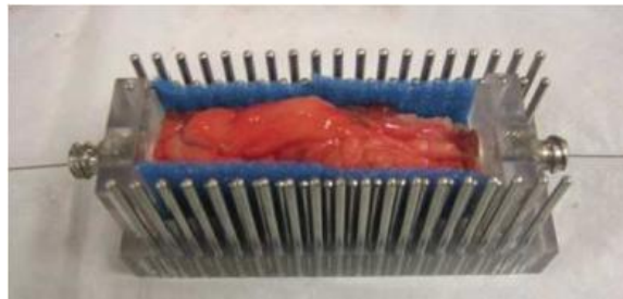
Figure 6.6.: Tissue cage fixture: The artery is fixed in the cage and an automatic pullback is performed in saline and human blood. The histology sections are taken at every 2 mm using side rods after the artery was fixed by formaldehyde [38].
