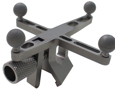
Figure 5.4.: Exemplary IR marker target. The IR reflecting markers are distributed in a way, such that no ambiguities arise when calculating the pose based on the relative distances.
