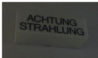
Figure 11.7.: Example of way of warning the presence of invisible radiation. Sign on door turns on when radiation is been applied. Also sound is made to make personnel aware of danger.
