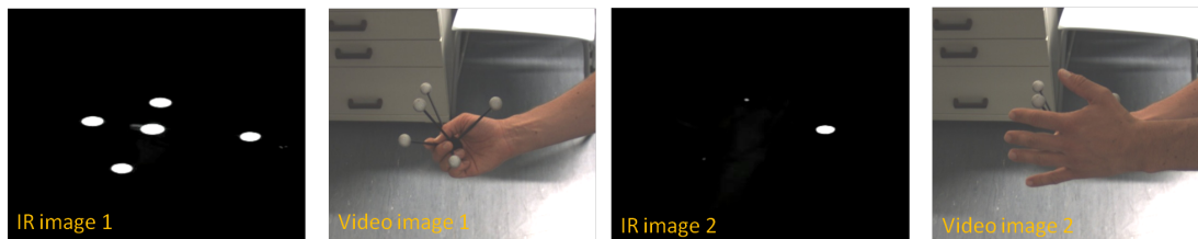
Figure 7.6.: Example of advantage of configuration where optical camera and tracking volume overlap. In images 1 no occlusion is present and optical image and tracking image (IR image) show all balls of the tracking target. In the second image the IR image shows only one ball, but it is impossible to know what is occluding the rest of the tracking markers. This can be easily seen in the optical image taken from almost the same perspective.
