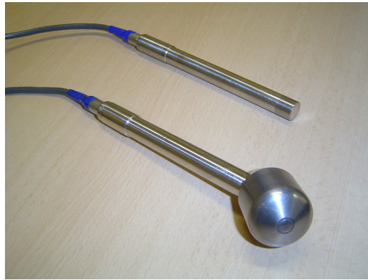
Figure 5.6.: High-energy and standard gamma-probes by Intra-Medical Imaging. The shielding of the high-energy gamma-probe is in this case 2.5 [cm] of tungsten compared to the 2 [mm] shielding of the standard probe. The conventional gamma-probe has been designed for 140 [keV] (140 [keV] is the main energy emission peak of ^{99m}\text{Tc} , the standard radioactive label for SPECT and sentinel lymph-nodes applications.).
