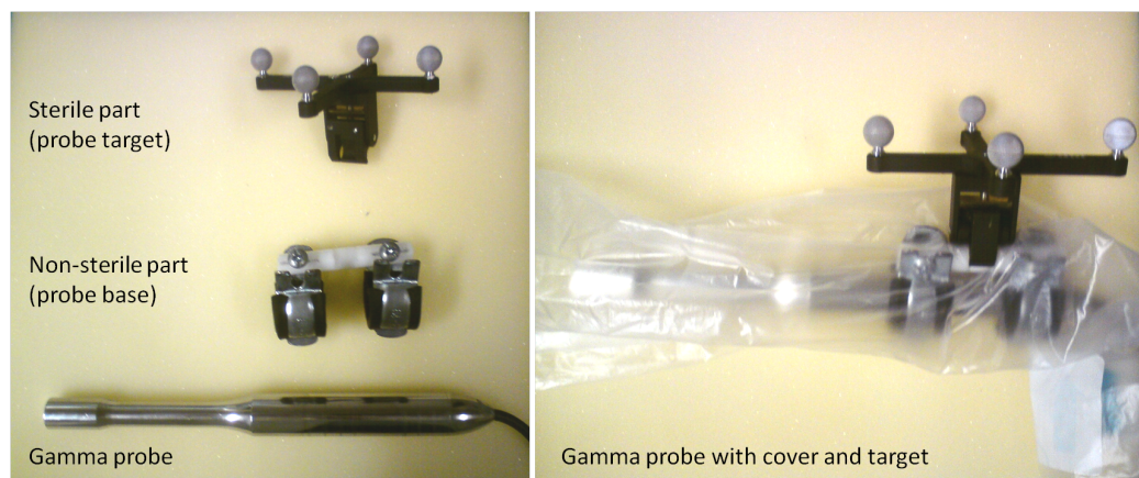
Figure 7.9.: Proposed solution for probe target including a fixed base that enables to keep the calibration between probe tip and tracking target constant while making possible the use of a sterile target over the sterile cover.
