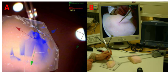
Figure 4.1.: Augmented reality visualization of the acquired activity of a phantom's surface beta activity. Blue is high measured activity, white is low. The upper number shows the measures of the real beta probe (which was turned off after acquisition), the lower number shows the simulated activity at the tip of the instrument. On the right side the same scene as on the left is seen from outside showing the simulated activity with the beta probe control unit turned off [364].
