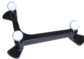
Figure 7.10.: Final version of patient target/reference. Three tracking markers are sufficient for tracking a 3D body. Dimensions are minimized in order to enable flexible positioning. Feet can be used to fix it to the patient with sterile tape.
