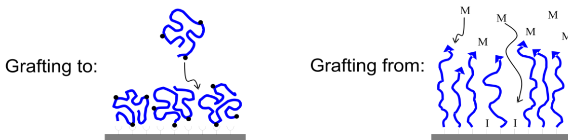
Figure 13. Schematic illustration of polymer brushes with different grafting densities prepared by ‘grafting to’ and ‘grafting from’ methods (From Ref. [66]).
