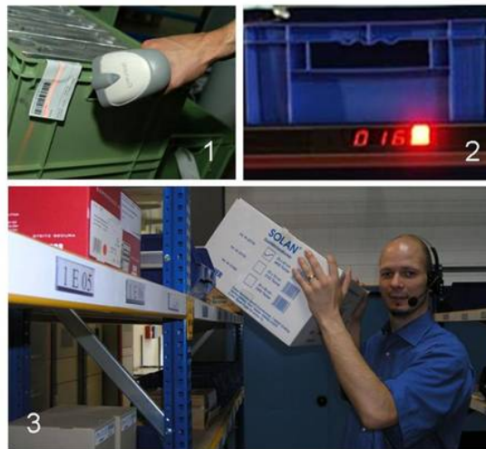
Figure 2.2.: Common order picking technologies: MDT with scanner (1), Pick-by-Light (2) and Pick-by-Voice (3). Courtesy of [127].
