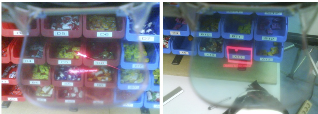
Figure 5.9.: The frame highlighting a box (photographed through the Nomad HMD). The frame is partly occluded by a virtual occlusion object of the shelf. The Frame is supported by the Compass-like Arrow visualization.
